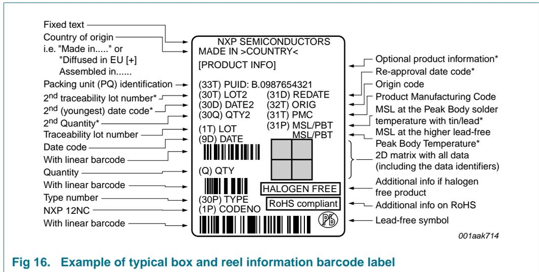
Fig 16. Example of typical box and reel information barcode label
