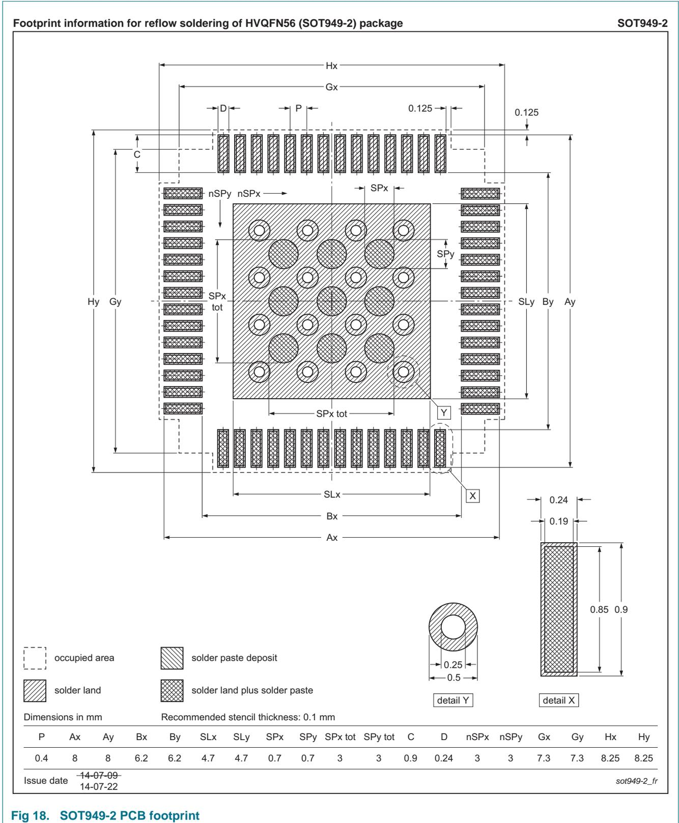
Fig 18. SOT949-2 PCB footprint
