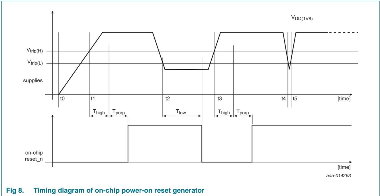
Fig 8. Timing diagram of on-chip power-on reset generator
