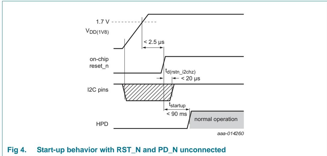
Fig 4. Start-up behavior with RST\_N and PD\_N unconnected
