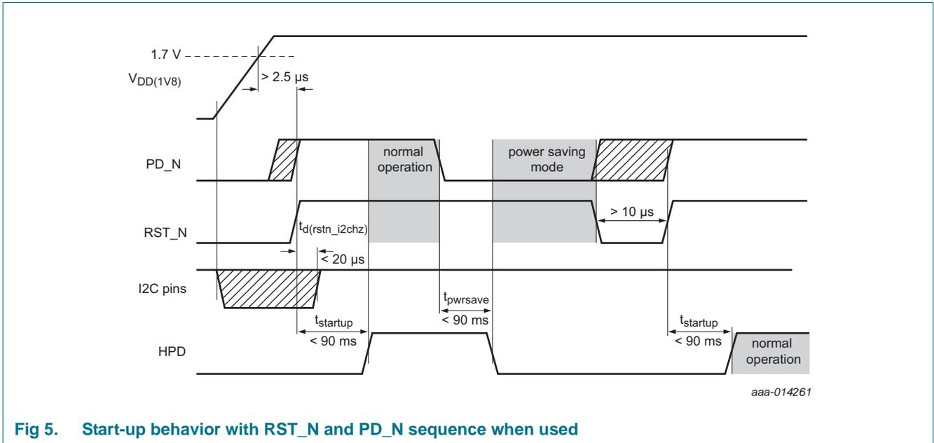
Fig 5. Start-up behavior with RST\_N and PD\_N sequence when used
