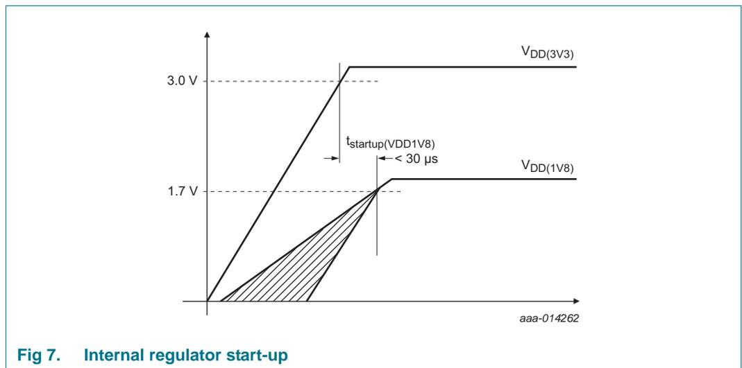
**Fig 7. Internal regulator start-up**
