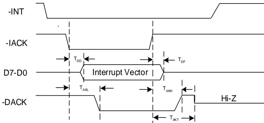
**Figure 7: Interrupt Timing**
