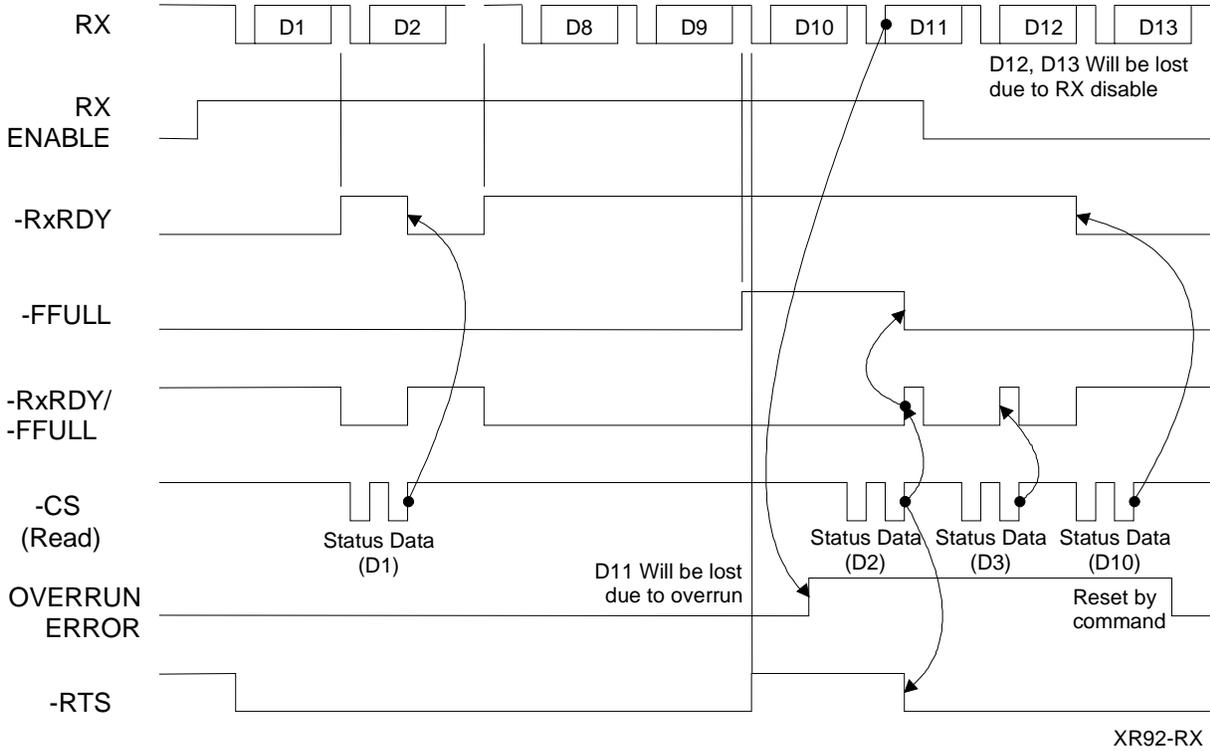
**Figure 8: Receive Timing**
