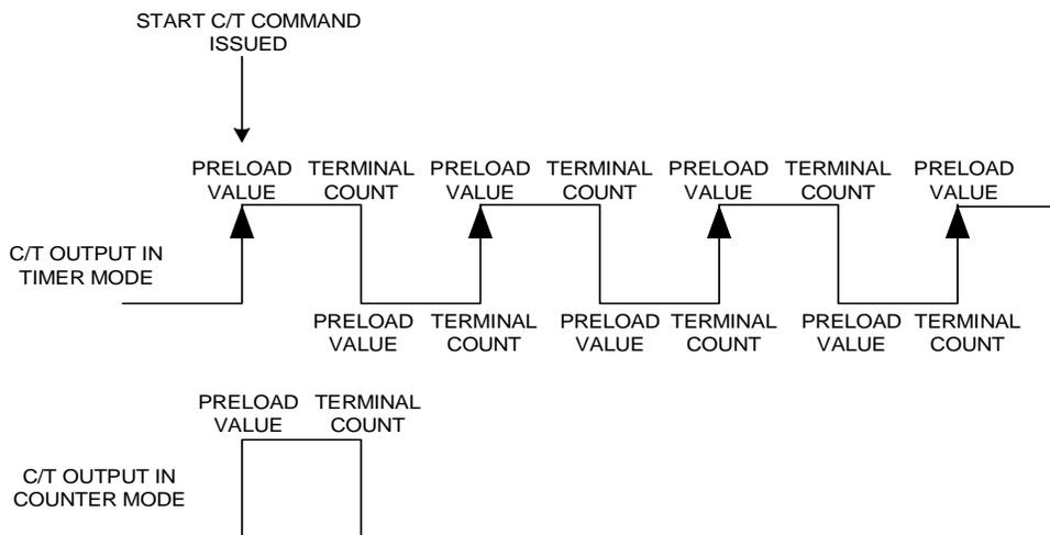
**Figure 2: C/T output in Timer and Counter modes.**
