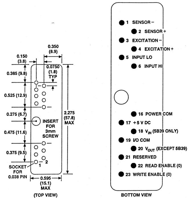
Figure 4 . Model 5B Series Module, with pin-out assignments.
