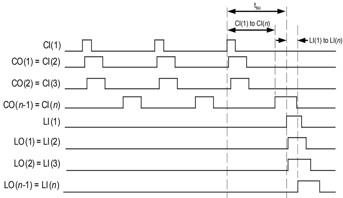
Figure 7. Signal Delay Mismatch Timing Diagram.  $t_{su}$  is the setup time for signals (CI to LI) applied to the first pixel in the chain. Note the difference in delay for CI(1) to CI(n) compared to the delay for LI(1) to LI(n). This must be compensated by increasing  $t_{su}$ .
