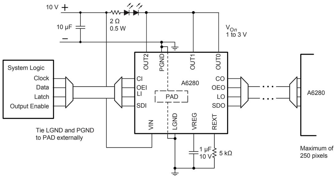
Figure 9. Application Driving High Power LED at 450 mA
