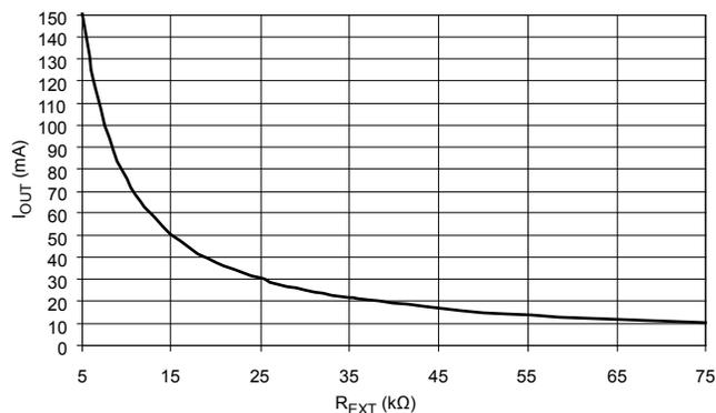
Figure 5. Output Current versus External Resistor,  $R_{EXT}$
