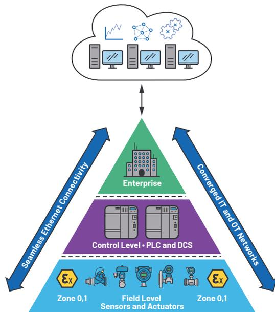
Figure 1. Seamless Ethernet connectivity to process automation field sensors and actuators.
