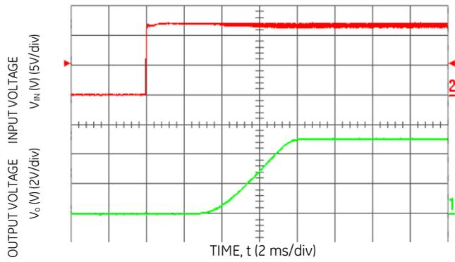
**Figure 16. Typical Start-Up with application of  $V_{in}$  with low-ESR polymer capacitors at the output ( $7 \times 150\ \mu\text{F}$ ) ( $V_{in} = 12\text{ Vdc}$ ,  $V_o = 5.0\text{ Vdc}$ ,  $I_o = 10\text{ A}$ ,  $C_o = 1050\ \mu\text{F}$ )**
