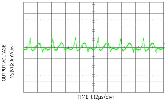
**Figure 9. Typical Output Ripple and Noise**
