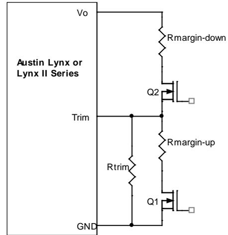
**Figure 29. Circuit Configuration for margining Output voltage.**
