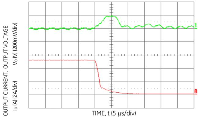
**Figure 11. Transient Response to Dynamic Load Change**
