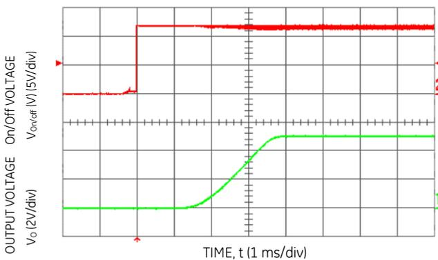
**Figure 15. Typical Start-Up Using Remote On/Off with Low-ESR external capacitors ( $C_o = 5000\ \mu\text{F}$ ) ( $V_{in} = 12.0\text{ Vdc}$ ,  $V_o = 5.0\text{ Vdc}$ ,  $I_o = 10.0\text{ A}$ ,  $C_o = 1050\ \mu\text{F}$ ).**
