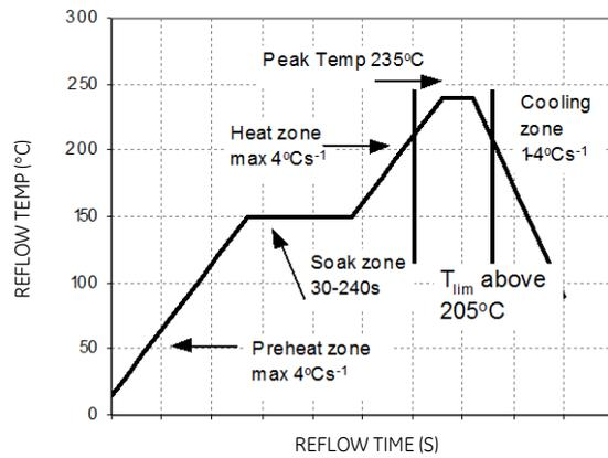
Figure 34. Reflow Profile for Tin/Lead (Sn/Pb) process.
