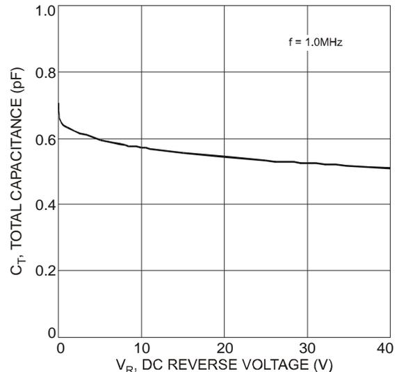
Fig. 4 Total Capacitance vs. Reverse Voltage, Per Element
