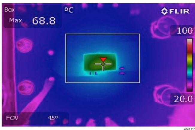
Figure 10. LTM4647 12V<sub>IN</sub> to 1V<sub>OUT</sub> at 30A with No Air Flow and No Heat Sink
