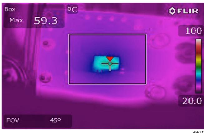
Figure 11. LTM4647 12V<sub>IN</sub> to 1V<sub>OUT</sub> at 30A with 200LFM Air Flow and No Heat Sink
