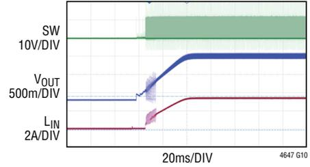
$V_{IN} = 12V$ ,  $V_{OUT} = 1.2V$ ,  $F_S = 500kHz$ , NO LOAD
