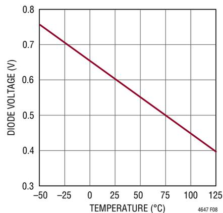
Figure 8. Diode Voltage  $V_D$  vs Temperature  $T(^{\circ}\text{C})$
