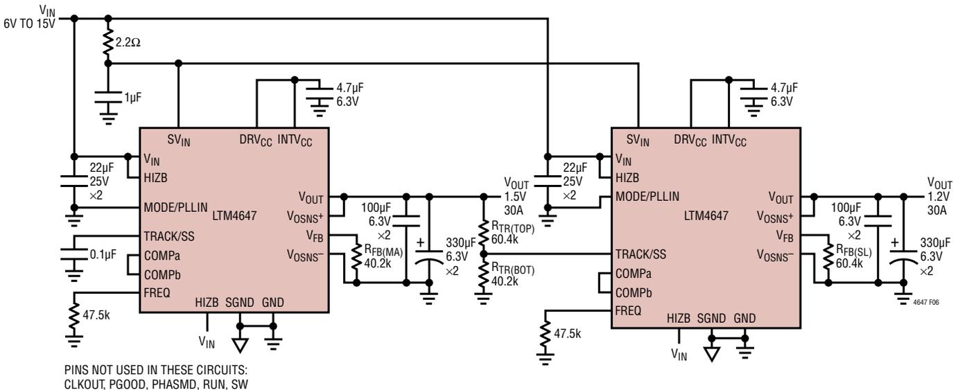
Figure 6. Example Schematic of Ratiometric Output Voltage Tracking
