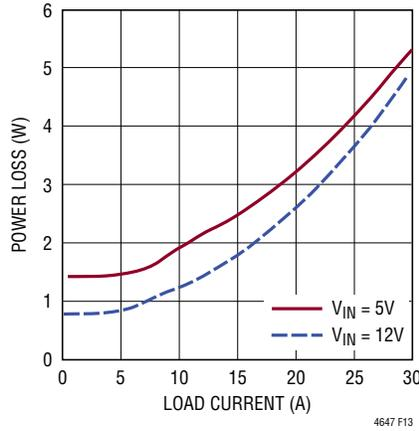
Figure 13. 1.5V Power Loss Curve
