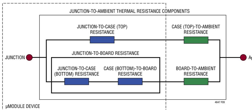
Figure 9. Graphical Representation of JESD51-12 Thermal Coefficients
