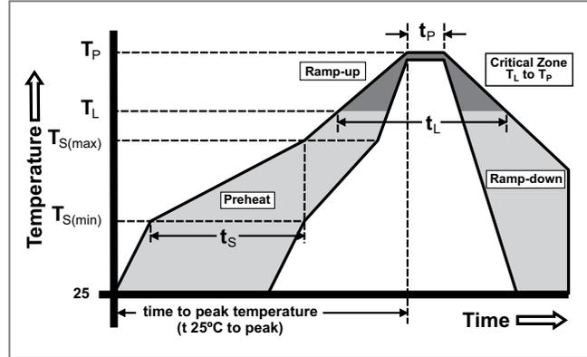
**Soldering Parameters - Wave Soldering (Thru-Hole Devices)**
