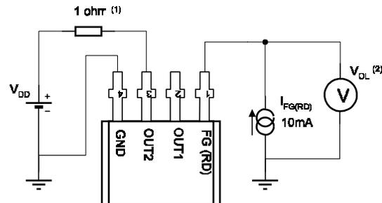
Note 1 - The chip is triggered to have OUT2 = high and OUT1 = low. A small resistor value is used to have  $V_{DD}$  equal to  $V_{OUT2}$
