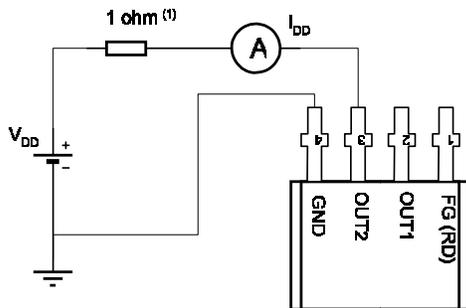
Note 1 - The chip is triggered to have OUT2 = high and OUT1 = low. A small resistor value is used to have  $V_{DD}$  equal to  $V_{OUT2}$
