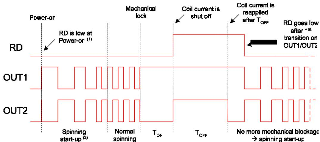
Note 1 : At Power-on, RD is low. If no transition occurs on OUT1/OUT2 before  $T_{ON}$  time, RD goes high.
