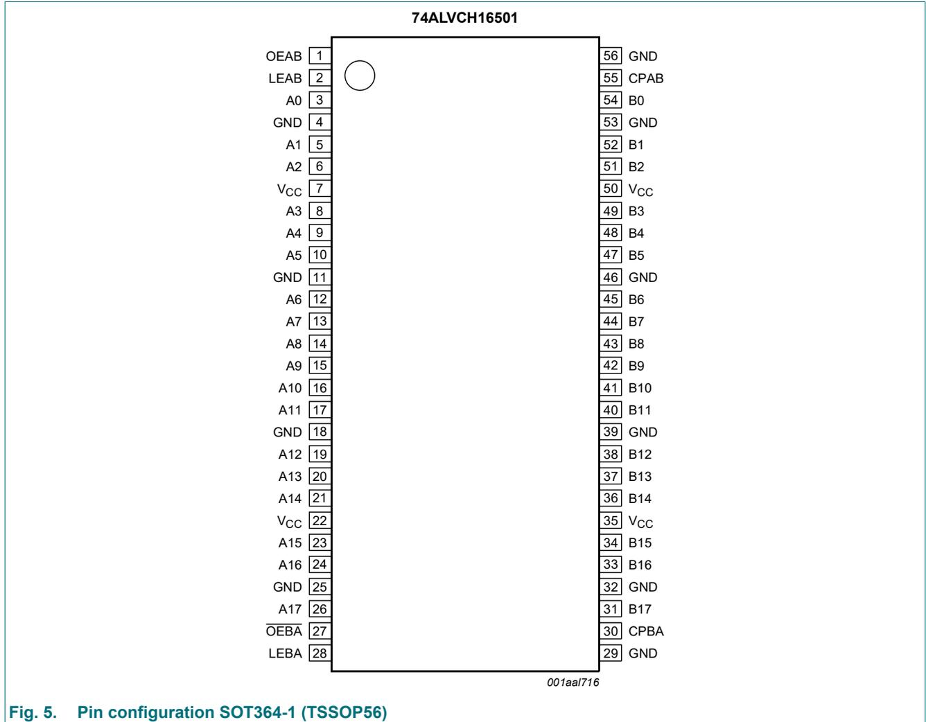
**Fig. 5. Pin configuration SOT364-1 (TSSOP56)**
