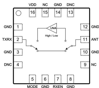
**Figure 1: Functional Block Diagram**
