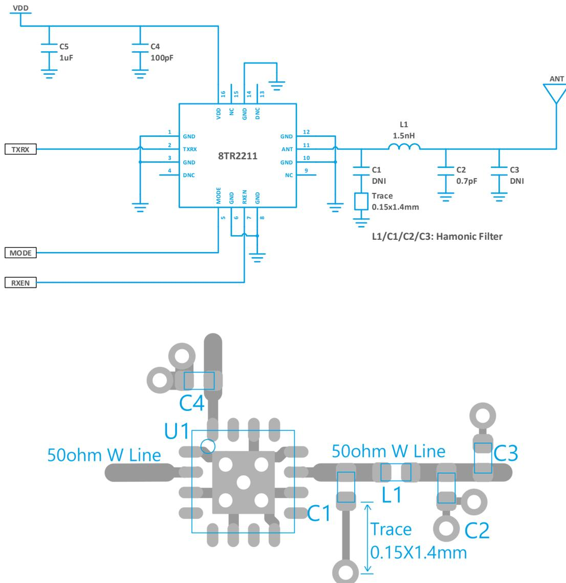
**Figure 4: 8TR2211 Reference Design Schematic and PCB Layout**
