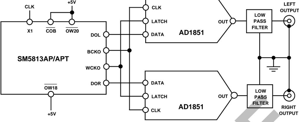
Figure 11. AD1851 with NPC SM5813AP/APT Digital Filter
