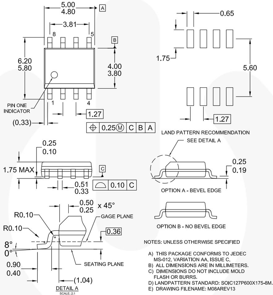
Figure 17. 8-Lead, SOIC, JEDEC MS-012, 150" NARROW BODY
