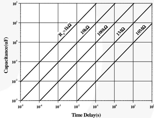
**Figure 3. Resistance and Capacitance vs. Time Delay ( $t_D$ )**
