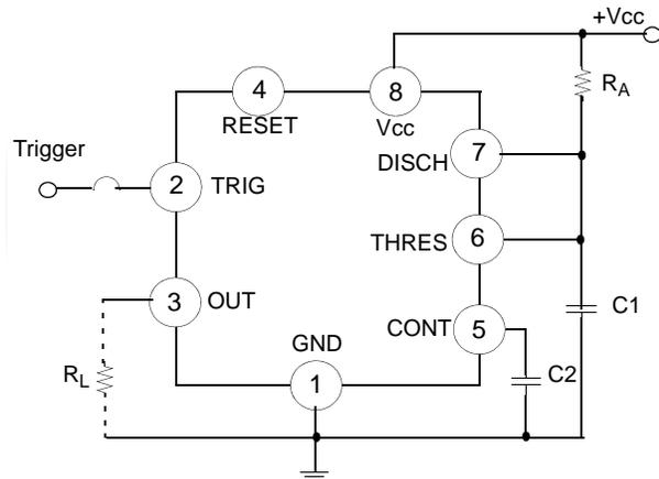
**Figure 2. Monostable Circuit**
