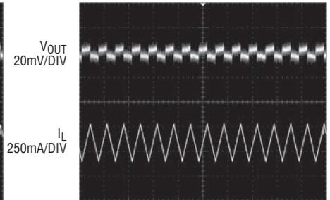
$V_{IN} = 3.6V$        $2\mu\text{s/DIV}$       3417A-2 G03
