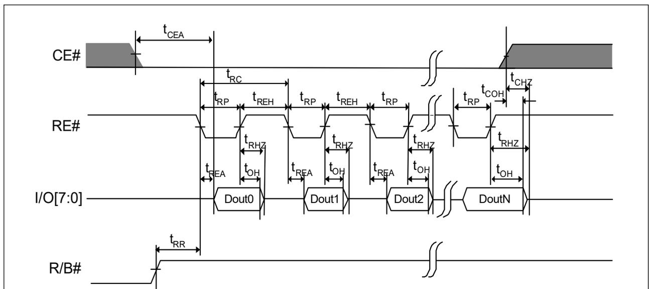
**Figure 9-2. AC Waveforms for Sequential Data Out Cycle (After Read) - EDO Mode**
