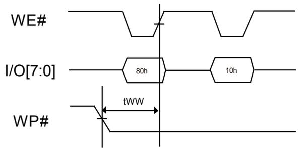
**Figure 47-3. Enable Erasing of WP# Signal**
