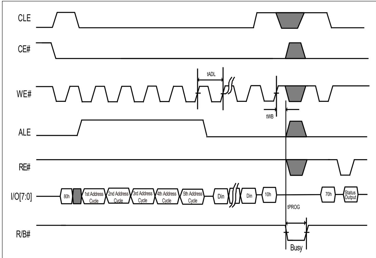
Figure 33. AC Waveforms for OTP Data Program with Random Data Input
