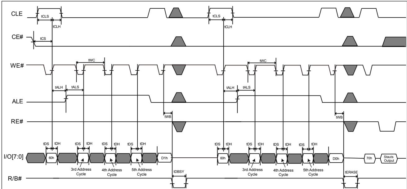
**Figure 40. AC waveforms for Two-plane Program (Traditional)**
