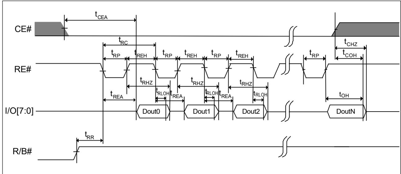
Figure 10. AC Waveforms for Random Data Output
