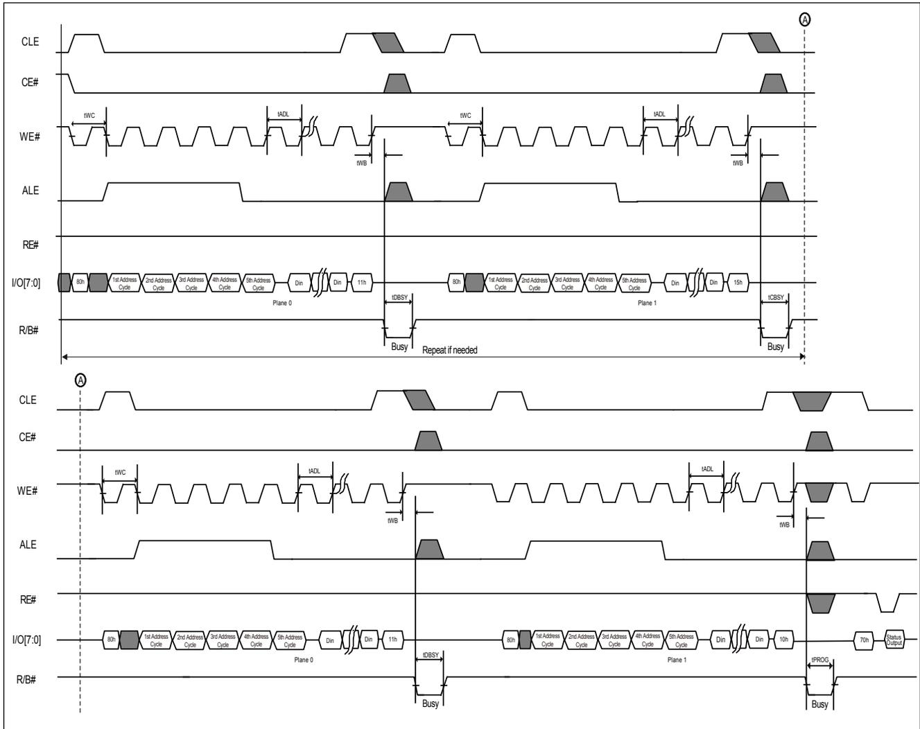
**Figure 39. AC Waveforms for Two-plane Erase (ONFI)**
