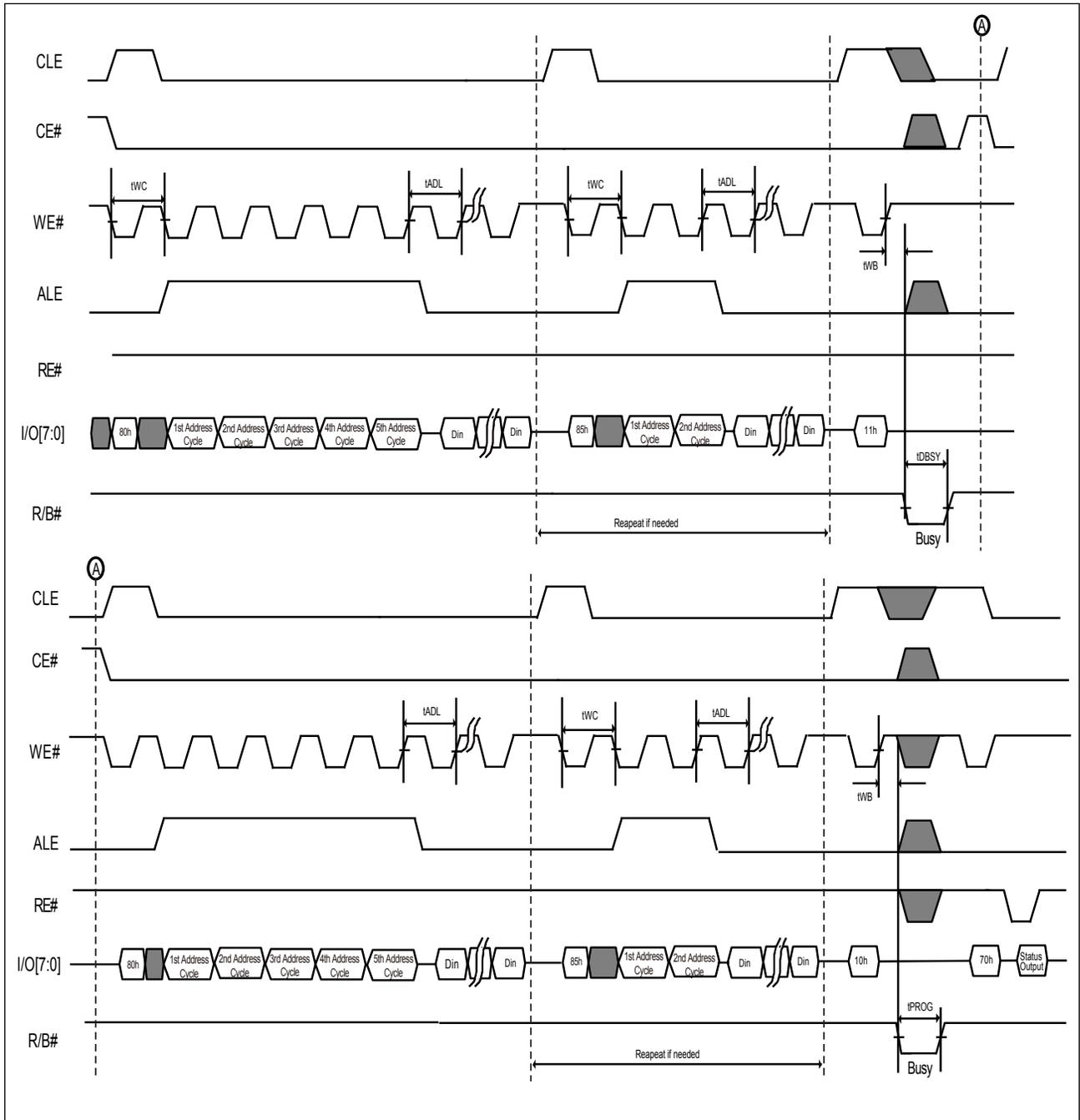
Figure 38. AC Waveforms for Two-plane Cache Program (ONFI)
