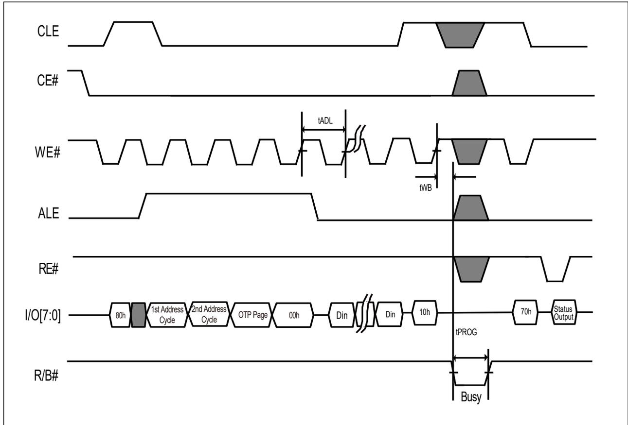
Figure 32-2. AC Waveforms for OTP Data Program (2Gb/4Gb)
