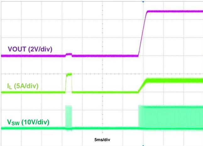
Figure 22. Output Short Recovery,  $I_{OUT} = 3.5\text{A}$
