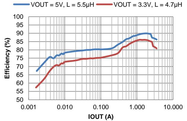
Figure 5. Efficiency vs. Output Current, VIN = 24V
