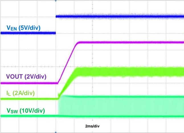
Figure 19. Startup Using EN,  $I_{OUT} = 3.5\text{A}$
