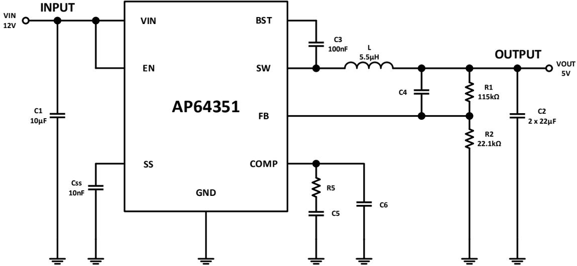
**Figure 27. Example Circuit for Loop Compensation Calculations**
