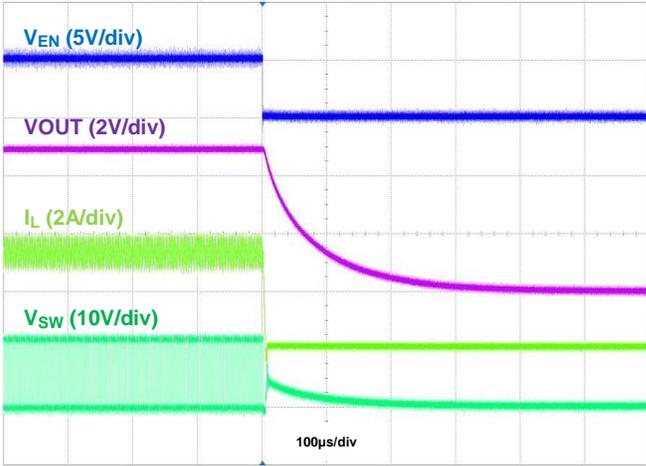
Figure 20. Shutdown Using EN,  $I_{OUT} = 3.5\text{A}$
