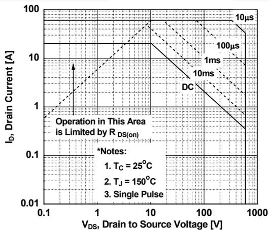
**Figure 10. Maximum Safe Operating Area for FCPF190N60E**
