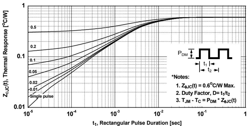
Figure 14. Transient Thermal Response Curve for FCPF190N60E
