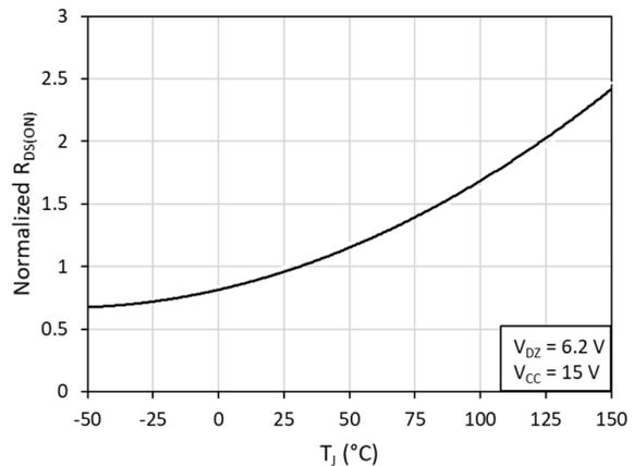
Fig. 8. Normalized on-resistance ( $R_{DS(ON)}$ ) vs. junction temperature ( $T_J$ )
