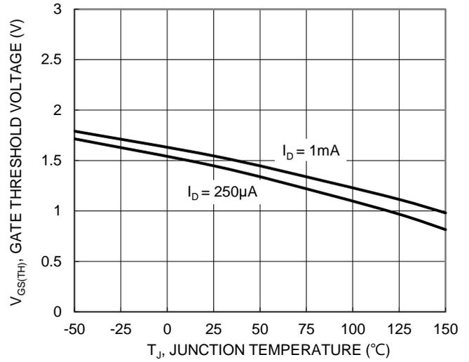
Figure 20. Gate Threshold Variation vs. Junction Temperature
