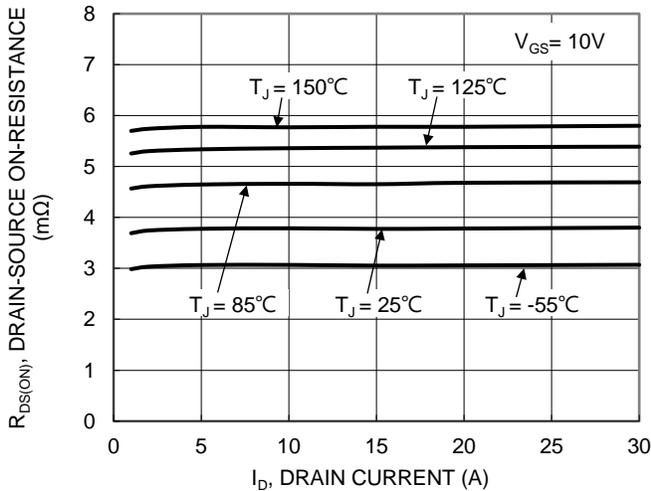
Figure 17. Typical On-Resistance vs. Drain Current and Temperature
