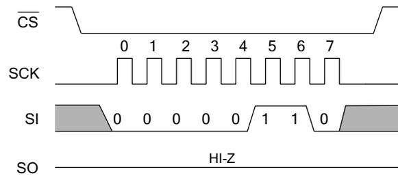
**WRDI - Reset Write Enable Latch**
