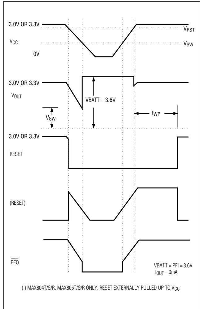
Figure 2. Timing Diagram
