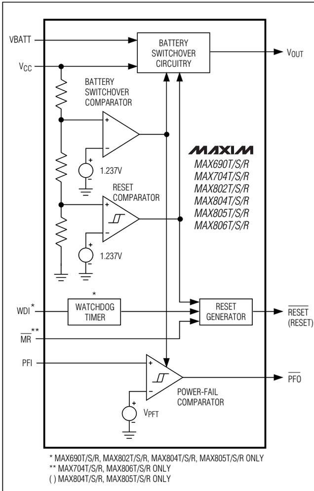
Figure 1. Block Diagram
