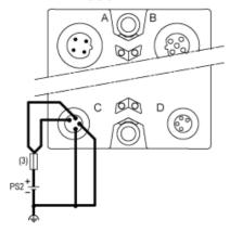
(3) External fuse, Type T slow-blow, 8 A max., 250 V PS2 External isolated I/O power supply, 24 Vdc
