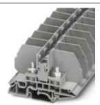
Bolt connection terminal block, Connection method: Bolt connection, Cross section: 2.5 mm² - 35 mm², AWG: 12 - 2, Width: 17 mm, Height: 48.6 mm, Color: gray, Mounting type: NS 35/7,5, NS 35/15
