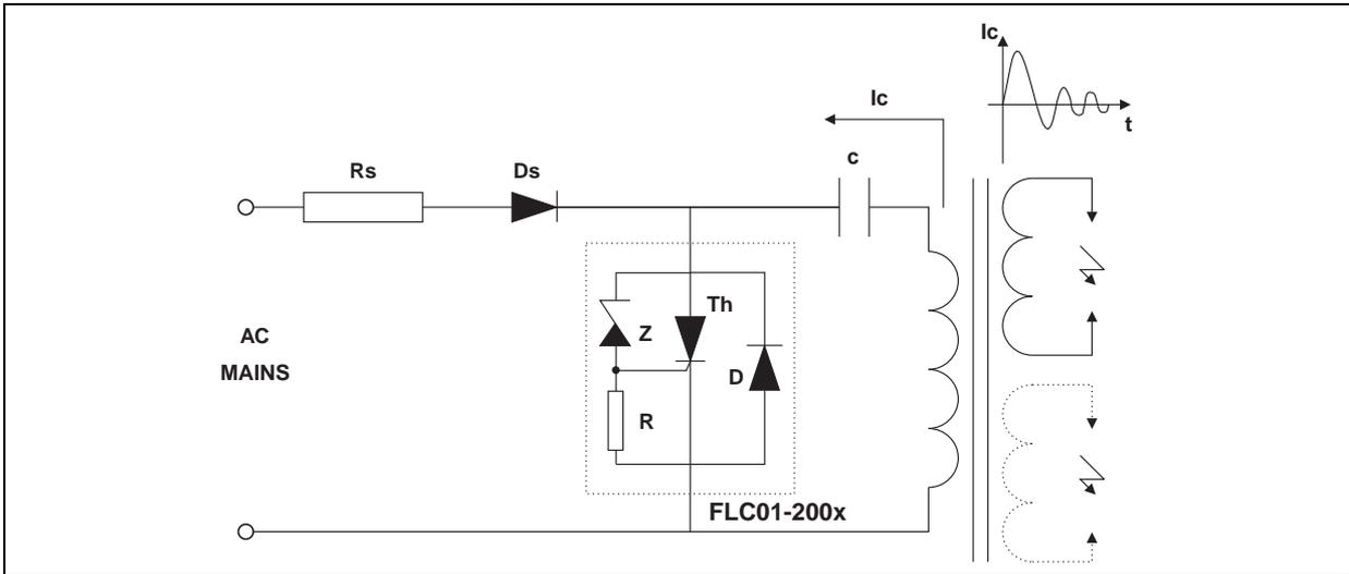
The applications of the lighter using the capacitance discharge topology operate in 2 phases:
