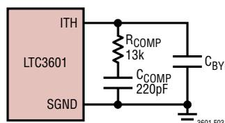
Figure 3. Compensation Components
