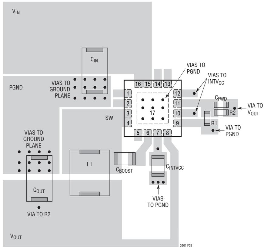
Figure 5. QFN Layout Example
