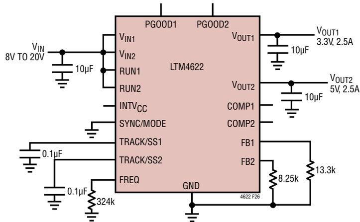
Figure 26. 8V<sub>IN</sub> to 20V<sub>IN</sub>, 3.3V and 5V Output at 2.5A with 2MHz Switching Frequency
