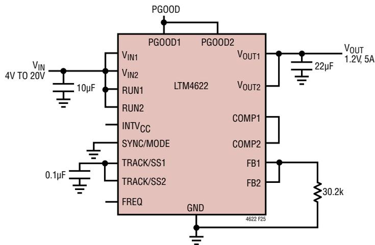
Figure 25. 4V<sub>IN</sub> to 20V<sub>IN</sub>, 1.2V Two Phase in Parallel 5A Design
