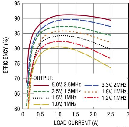
**Efficiency vs Load Current at 3.3V<sub>IN</sub>**
