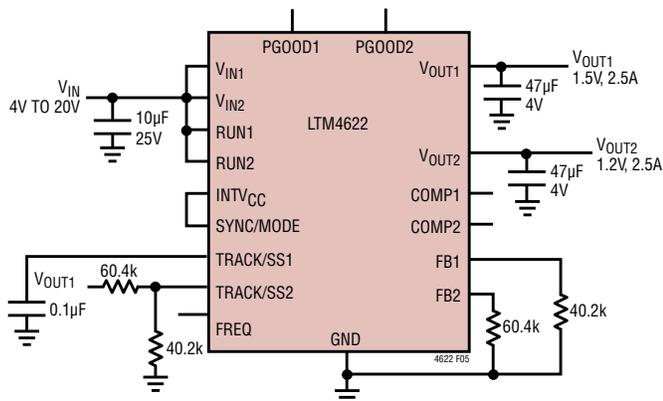
Figure 5. Example Schematic of Ratiometric Output Voltage Tracking
