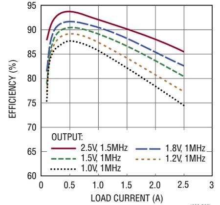
**Burst Mode Efficiency, 12V<sub>IN</sub>, 1.5V<sub>OUT</sub>**
