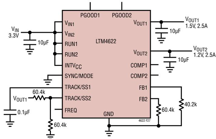
Figure 27. 3.3V<sub>IN</sub>, 1.5V and 1.2V Output at 2.5A Design with Output Coincident Tracking
