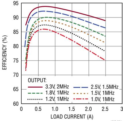
**Efficiency vs Load Current at 12V<sub>IN</sub>**
