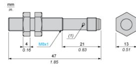
(1) LED, 4 viewing ports at 90° Note Fixing nut tightening torque : <2N.m
