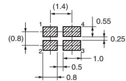
Unless otherwise specified, the dimensional tolerance is ± 0.1 mm.
