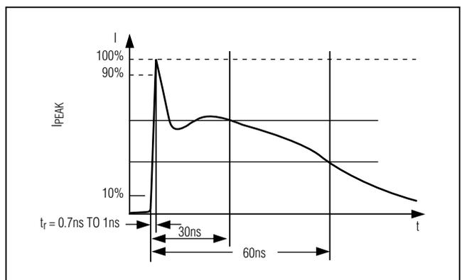
Figure 14. IEC 61000-4-2 ESD Generator Current Waveform
