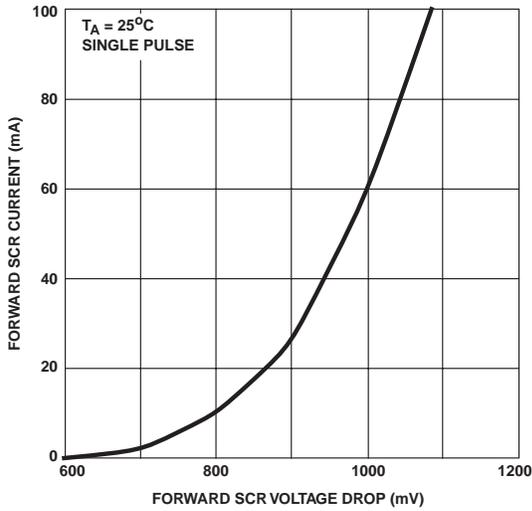
FIGURE 2. LOW CURRENT SCR FORWARD VOLTAGE DROP CURVE
