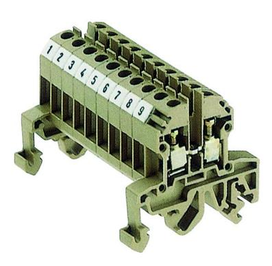
Feed-through terminal/block variant, Screw connection, Mounting type:Mounting rail TS 35/7.5 and TS 32, Rated cross-section: 4 mm², Colour: Beige
