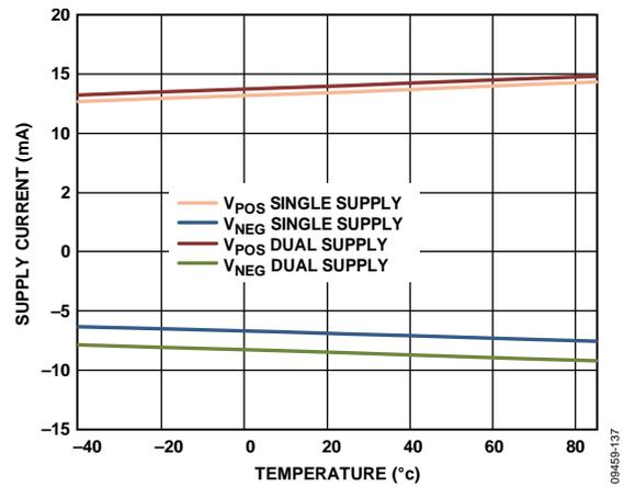
Figure 37. Supply Current vs. Temperature ( $V_{POS}$ ,  $V_{NEG}$ )
