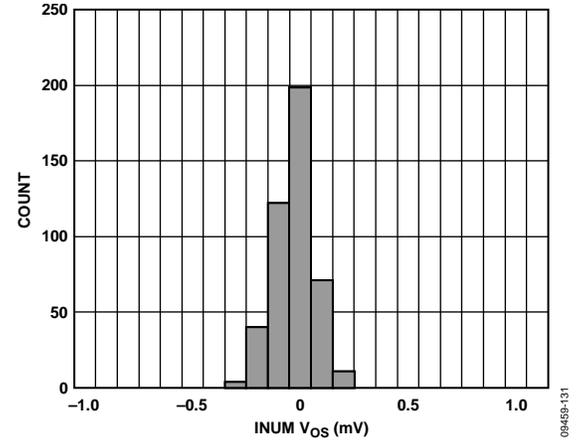
Figure 31.  $(V_{NUM} - V_{SUM})$  Histogram at 25°C
