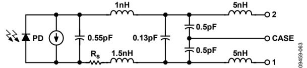
Figure 54. Photodiode Model
