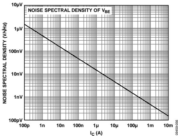
Figure 46. Noise Spectral Density of  $V_{BE}$  vs.  $I_C$
