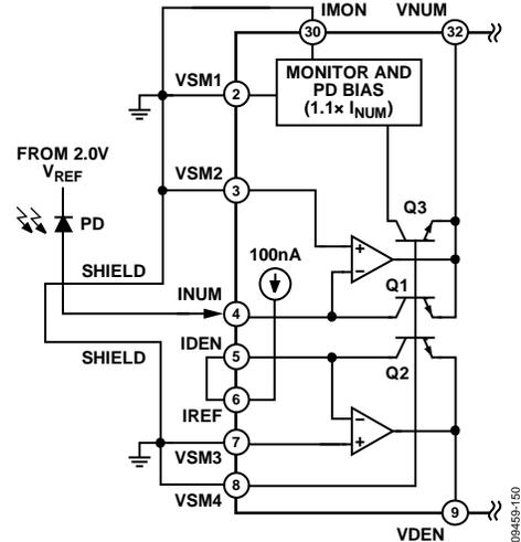
Figure 50. PD Bias with V<sub>SUM</sub> at Ground and Using 2.000 V
