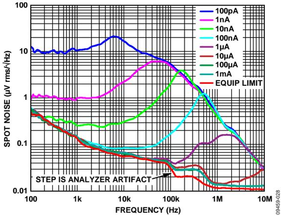
Figure 22. Spot Noise Spectral Density at  $V_{LOG}$  vs. Frequency for  $I_{NUM}$  in Decade Steps from 1 nA to 1 mA (Noise at lower frequencies, where NSD is flat, is limited by resistance used to generate dc  $I_{NUM}$  current. See the Noise vs. Current section for further explanation.)
