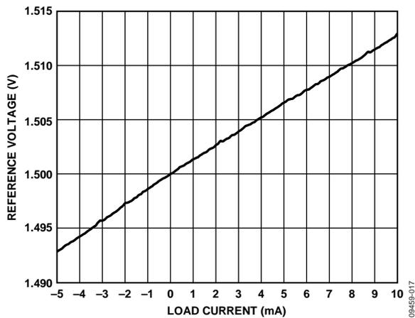
Figure 17. 1P5V vs. I<sub>LOAD</sub> (Positive Current Defined into 1P5V Pin)
