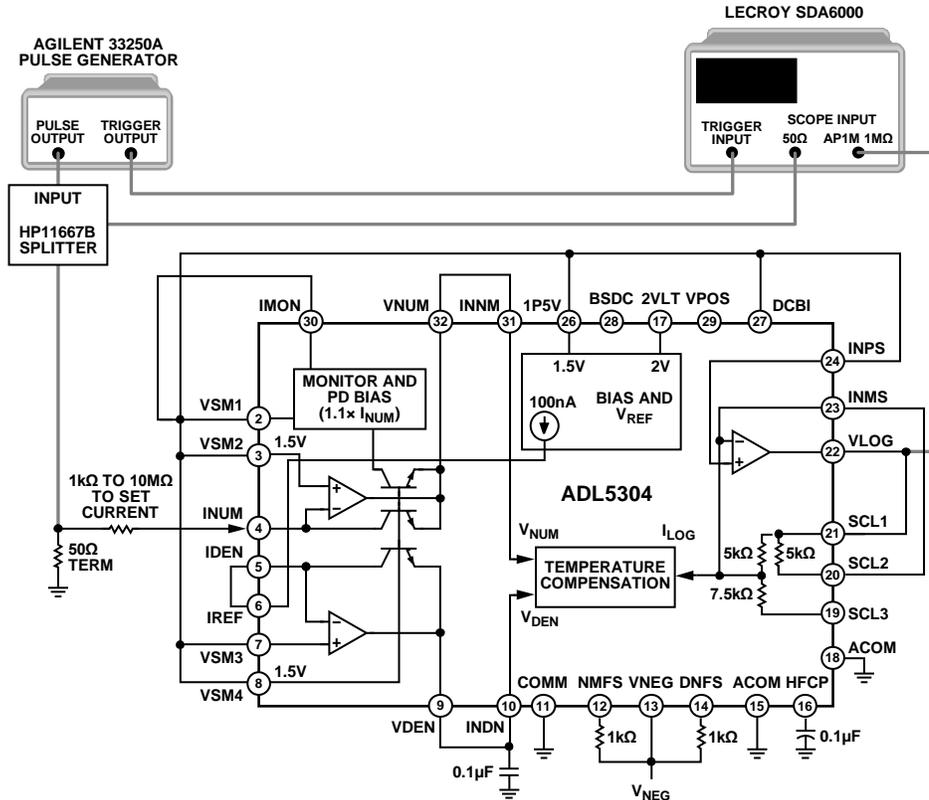
Figure 40. Setup for Measuring Pulse Settling
