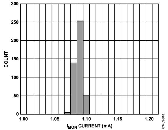
Figure 18. I<sub>MON</sub> Histogram at I<sub>NUM</sub> = 1 mA
