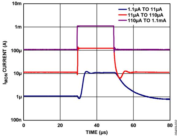
Figure 28.  $I_{MON}$  Pulse Response vs.  $I_{NUM}$
