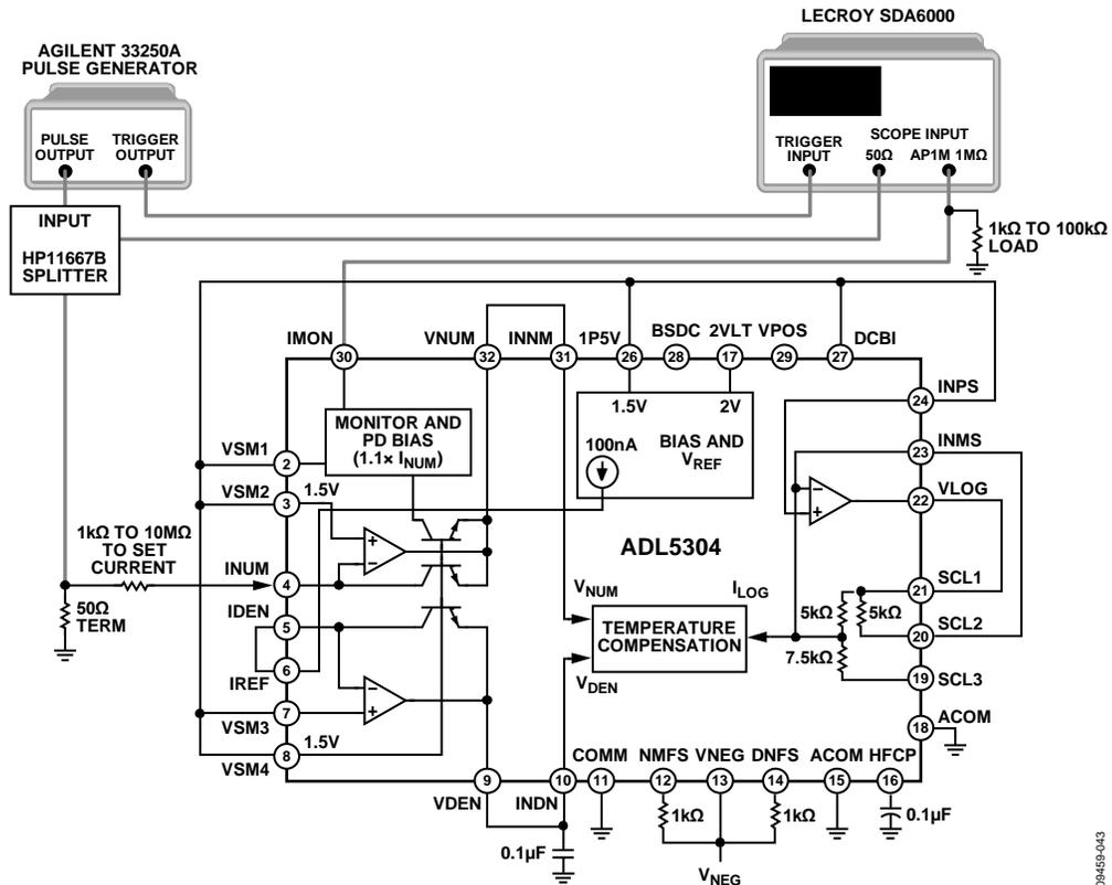
Figure 43. Setup for Measuring IMON Pulse Response
