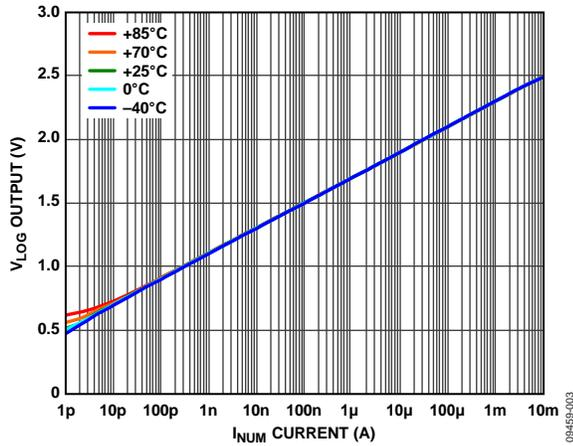
Figure 3.  $V_{LOG}$  vs.  $I_{NUM}$  for Multiple Temperatures
