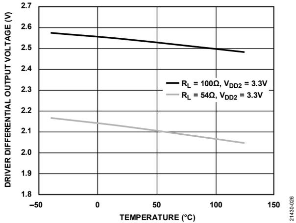
Figure 19. Driver Differential Output Voltage vs. Temperature
