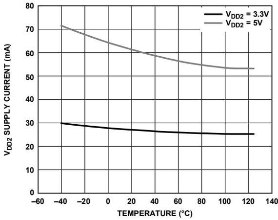
Figure 12. V<sub>DD2</sub> Supply Current vs. Temperature, Data Rate = 500 kbps, No Load
