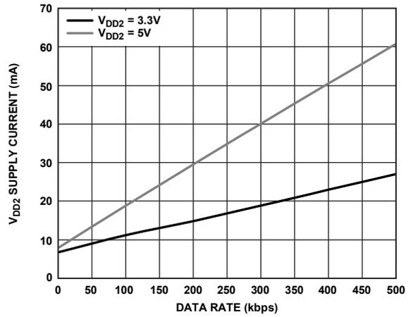
Figure 15. V<sub>DD2</sub> Supply Current vs. Data Rate, T<sub>A</sub> = 25°C, No Load
