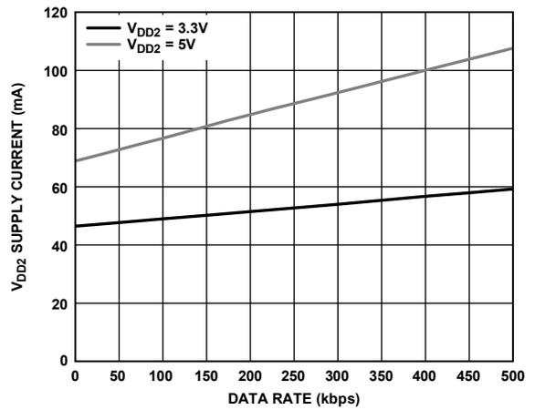
Figure 17. V<sub>DD2</sub> Supply Current vs. Data Rate, T<sub>A</sub> = 25°C, R<sub>L</sub> = 54Ω
