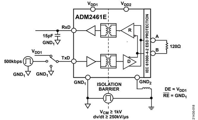
Figure 37. CMTI Test Diagram, Half-Duplex
