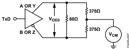
Figure 32. Driver Voltage Measurement over Common-Mode Range,  $|V_{OD3}|$
