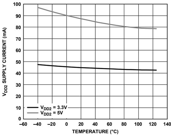
Figure 13. V<sub>DD2</sub> Supply Current vs. Temperature, Data Rate = 500 kbps, R<sub>L</sub> = 120Ω
