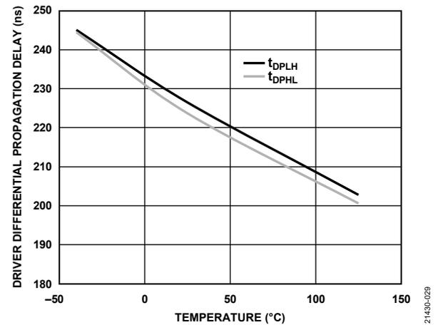
Figure 23. Driver Differential Propagation Delay vs. Temperature
