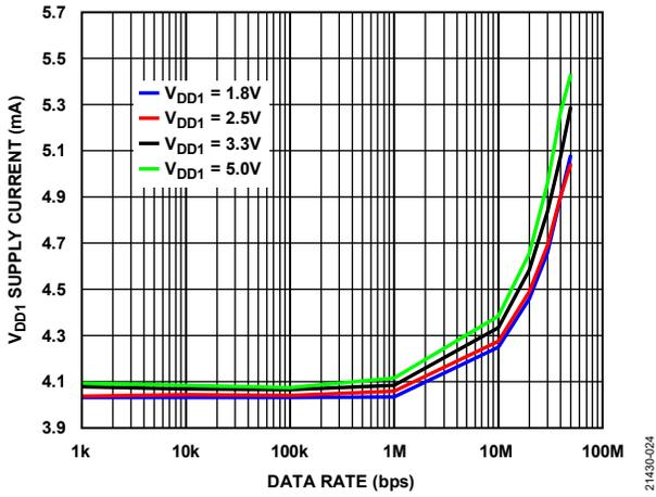
Figure 18.  $V_{DD1}$  Supply Current vs. Data Rate
