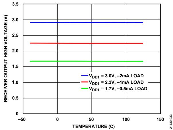
Figure 27. Receiver Output High Voltage vs. Temperature
