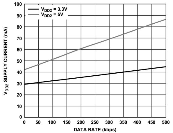
Figure 16. V<sub>DD2</sub> Supply Current vs. Data Rate, T<sub>A</sub> = 25°C, R<sub>L</sub> = 120Ω
