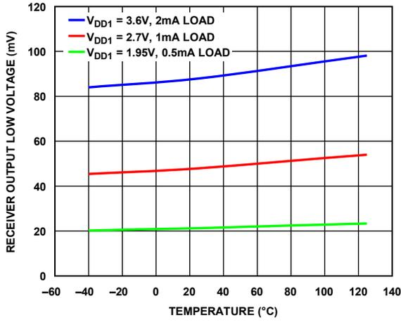
Figure 28. Receiver Output Low Voltage vs. Temperature
