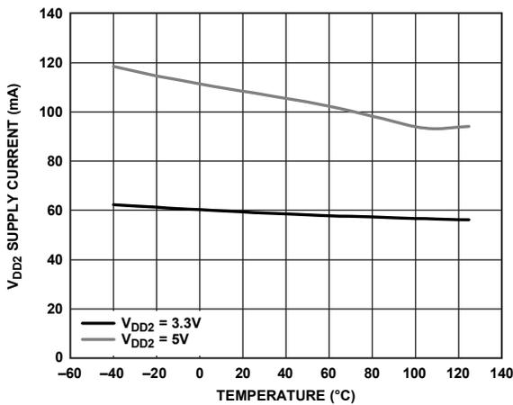
Figure 14. V<sub>DD2</sub> Supply Current vs. Temperature, Data Rate = 500 kbps, R<sub>L</sub> = 54Ω
