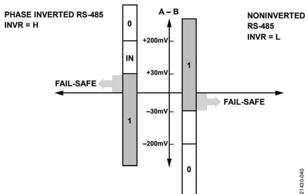
Figure 42. Noninverted RS-485 and Phase Inverted RS-485 Comparison
