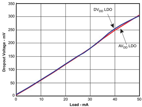
Figure 11. LDO Dropout Voltage vs Load Current
