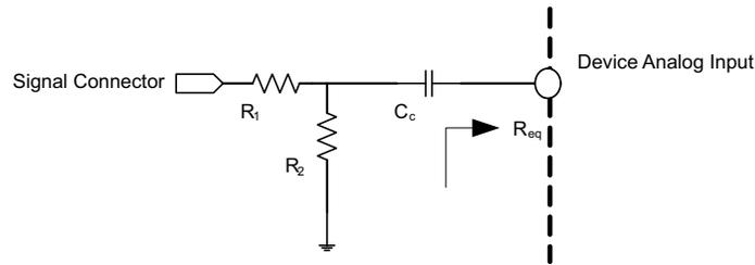
**Figure 21. Analog Input Connection With Resistor Divider Network**
