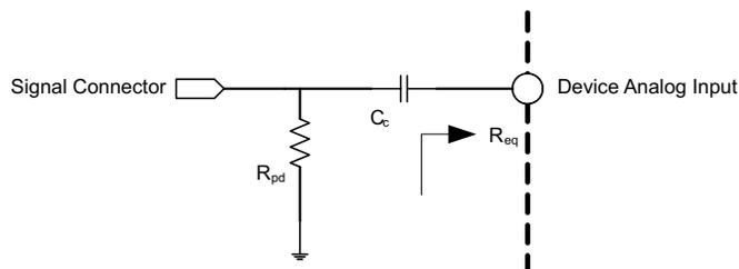
**Figure 20. Analog Input Connection With Pull-down Resistor**
