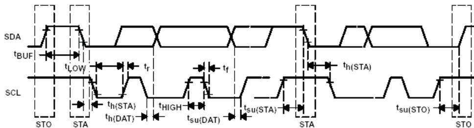
Figure 5. I<sup>2</sup>C Interface Timing
