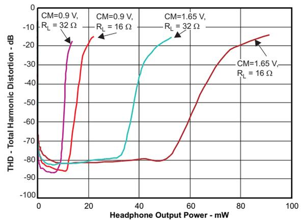
Figure 8. Total Harmonic Distortion vs Headphone Output Power
