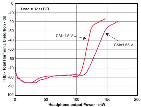
Figure 9. Total Harmonic Distortion vs Headphone Output Power
