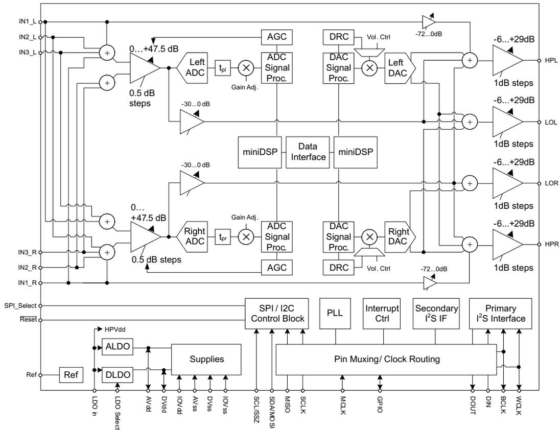
Figure 18. Block Diagram
