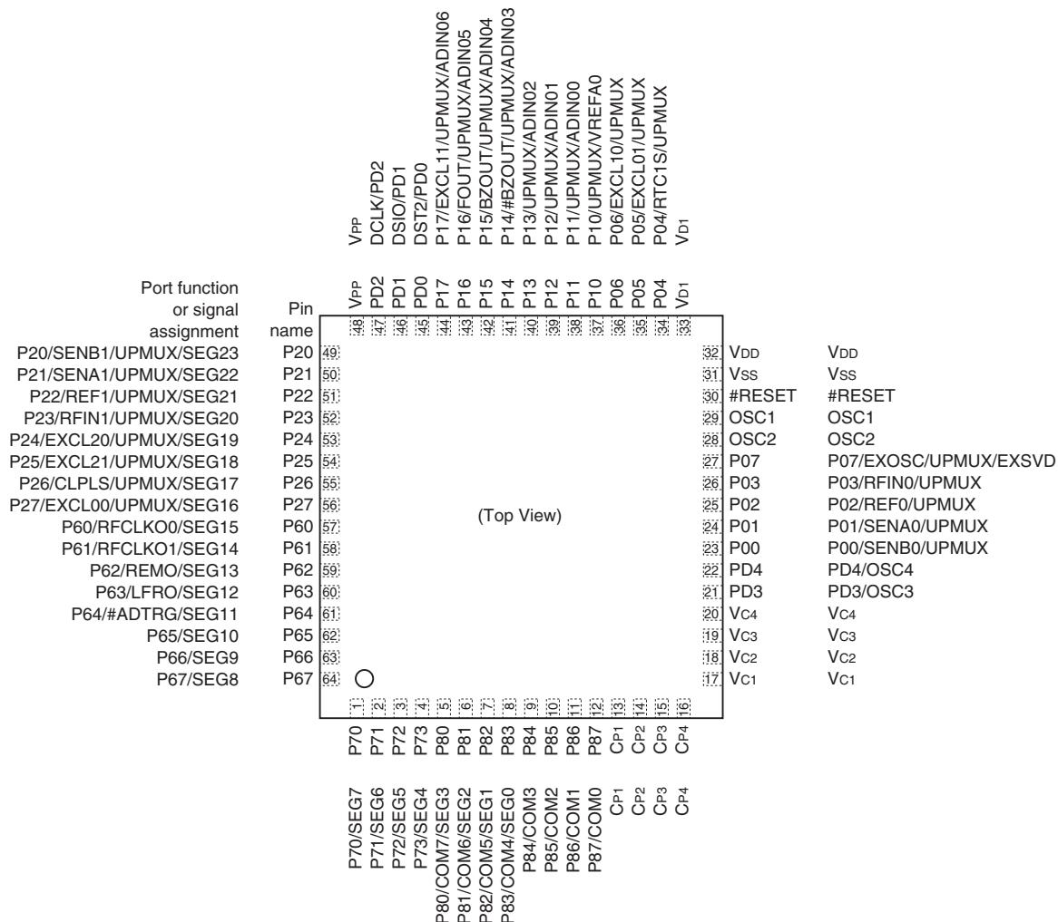
**Note:** The model in this package cannot be placed into super economy mode, as it does not have the VD2, Cv1, and Cv2 pins.
