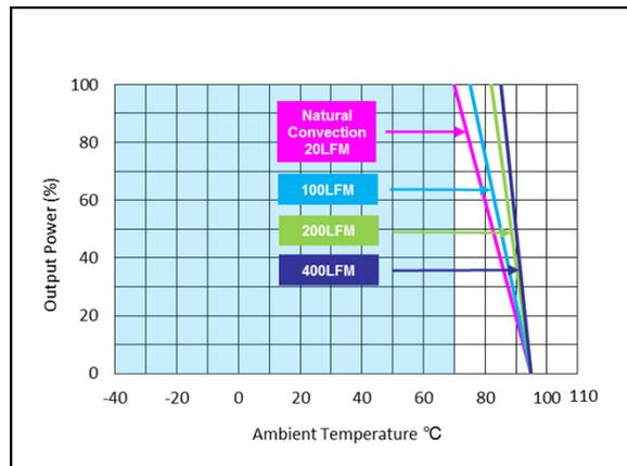
Figure 102: AEE01BB48-M Derating Curve (without heatsink)
