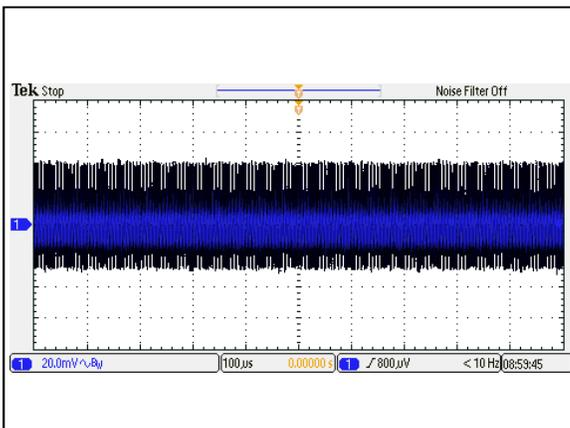
Figure 81: AEE01B48-M Ripple and Noise Measurement
