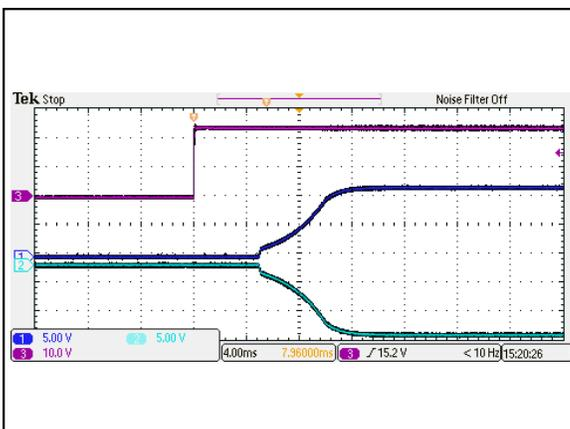
Figure 65: AEE01BB24-M Output Voltage Startup Characteristic by Vin
