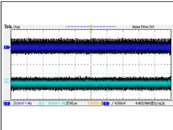
Figure 104: AEE01CC48-M Ripple and Noise Measurement
