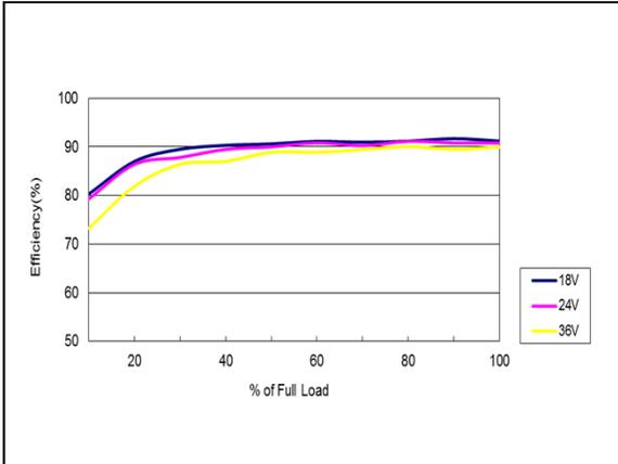
Figure 43: AEE01B24-M Efficiency Versus Output Current Curve
