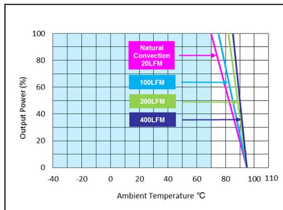
Figure 48: AEE01B24-M Derating Curve (without heatsink)
