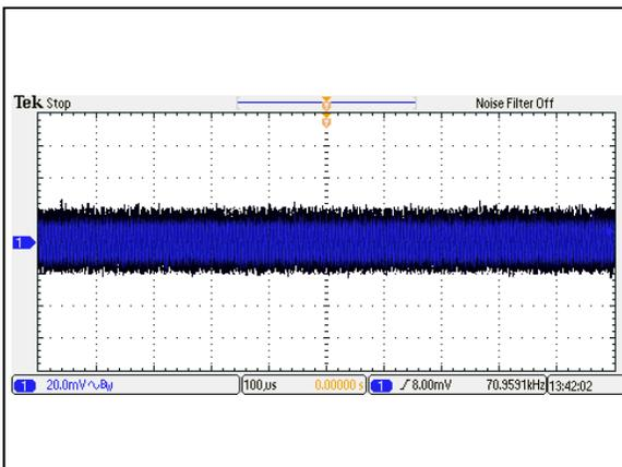
Figure 15: AEE01C12-M Ripple and Noise Measurement
