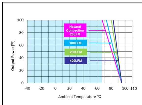
Figure 78: AEE03A48-M Derating Curve (without heatsink)
