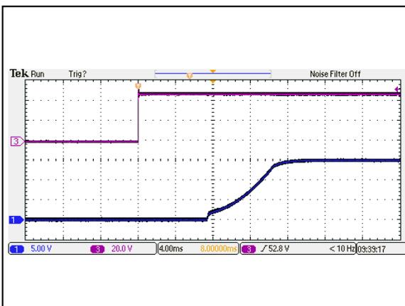
Figure 89: AEE01C48-M Output Voltage Startup Characteristic by Vin
