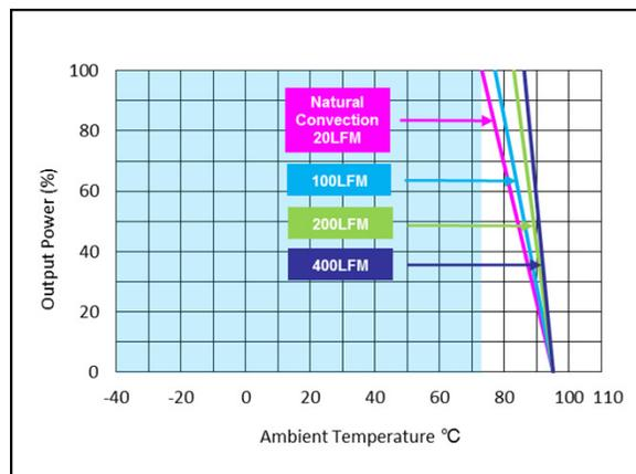
Figure 66: AEE01BB24-M Derating Curve (without heatsink)
