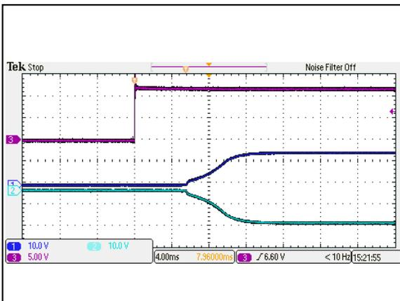
Figure 35: AEE01CC12-M Output Voltage Startup Characteristic by Vin
