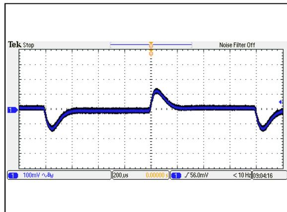
Figure 10: AEE01B12-M Transient Response
