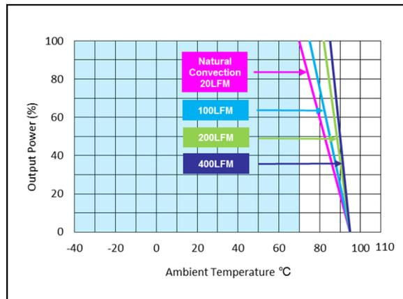
Figure 72: AEE01CC24-M Derating Curve (without heatsink)
