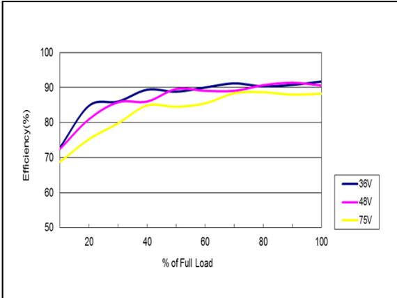
Figure 85: AEE01C48-M Efficiency Versus Output Current Curve
