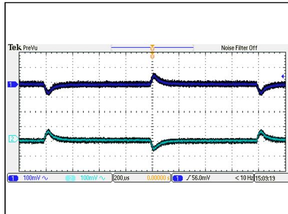
Figure 28: AEE01BB12-M Transient Response
