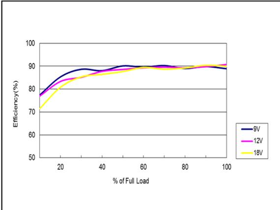
Figure 31: AEE01CC12-M Efficiency Versus Output Current Curve
