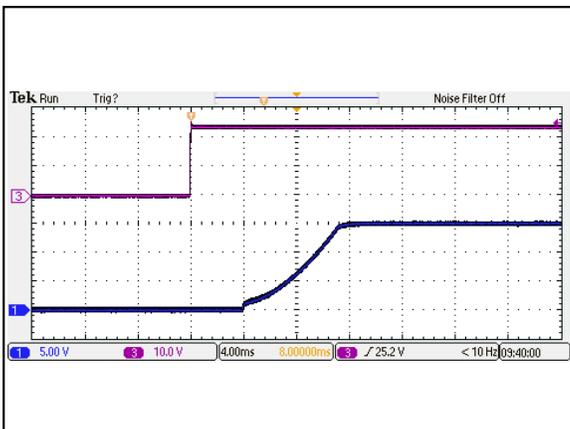
Figure 53: AEE01C24-M Output Voltage Startup Characteristic by Vin
