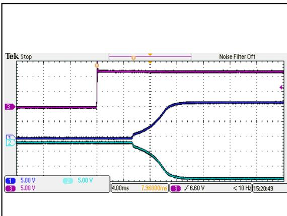
Figure 29: AEE01BB12-M Output Voltage Startup Characteristic by Vin
