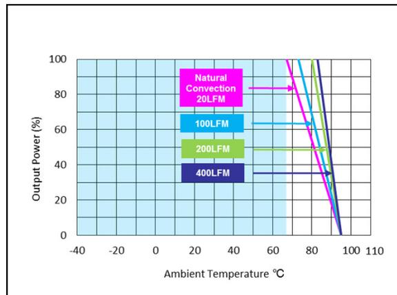
Figure 107: AEE01CC48-M Derating Curve (without heatsink)
