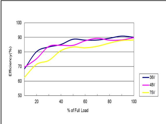
Figure 103: AEE01CC48-M Efficiency Versus Output Current Curve
