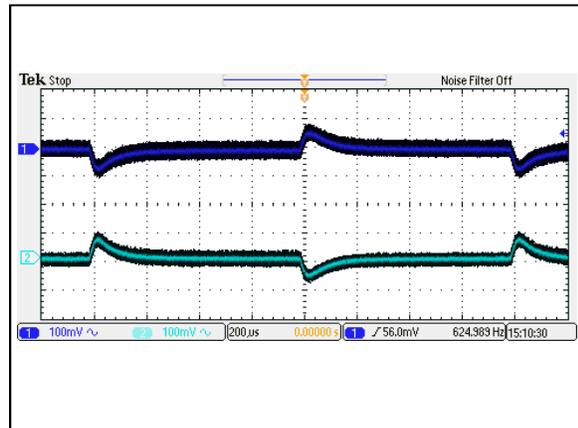
Figure 100: AEE01BB48-M Transient Response
