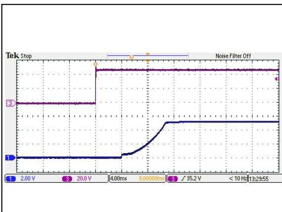
Figure 77: AEE03A48-M Output Voltage Startup Characteristic by Vin
