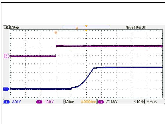
Figure 5: AEE03A12-M Output Voltage Startup Characteristic by Vin
