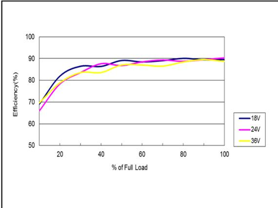
Figure 37: AEE03A24-M Efficiency Versus Output Current Curve
