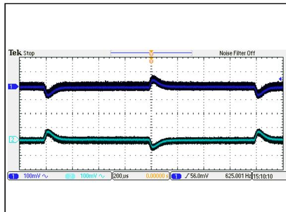
Figure 64: AEE01BB24-M Transient Response
