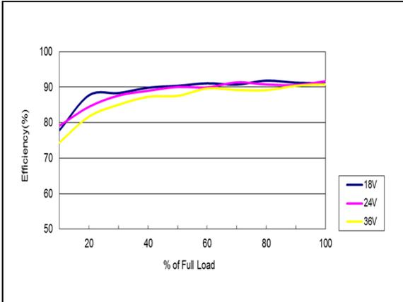
Figure 61: AEE01BB24-M Efficiency Versus Output Current Curve
