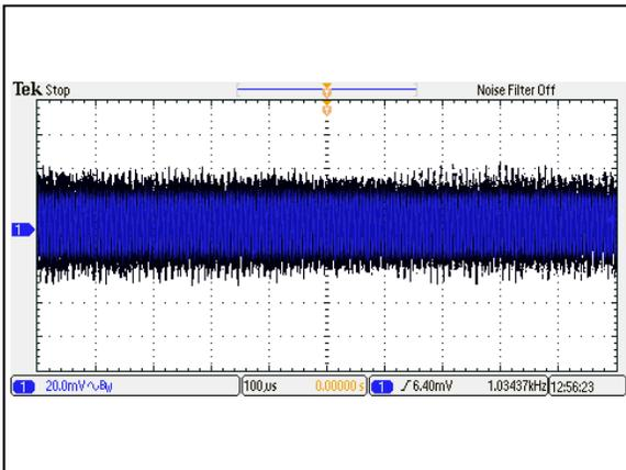
Figure 51: AEE01C24-M Ripple and Noise Measurement
