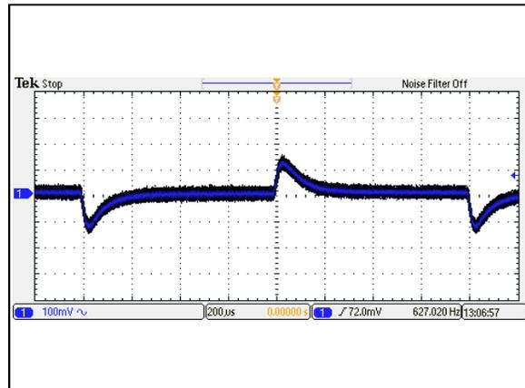
Figure 94: AEE01H48-M Transient Response
