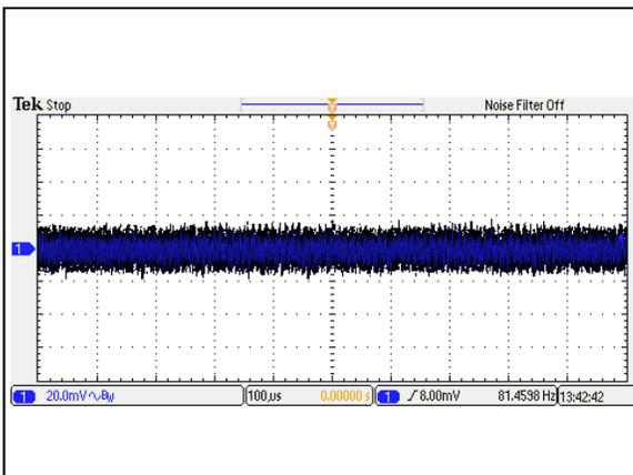
Figure 3: AEE03A12-M Ripple and Noise Measurement
