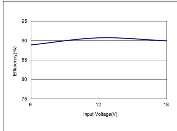
Figure 32: AEE01CC12-M Efficiency Versus Input Voltage Curve
