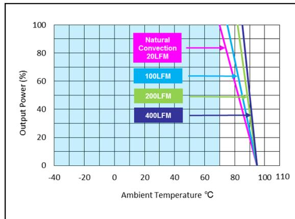
Figure 36: AEE01CC12-M Derating Curve (without heatsink)
