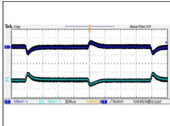
Figure 70: AEE01CC24-M Transient Response
