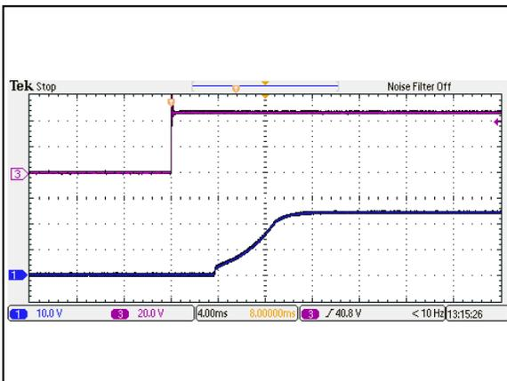
Figure 95: AEE01H48-M Output Voltage Startup Characteristic by Vin
