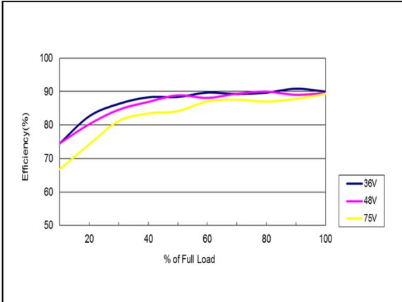
Figure 73: AEE03A48-M Efficiency Versus Output Current Curve
