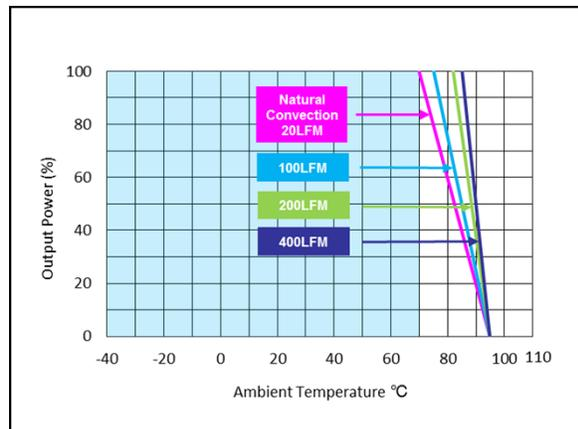
Figure 96: AEE01H48-M Derating Curve (without heatsink)
