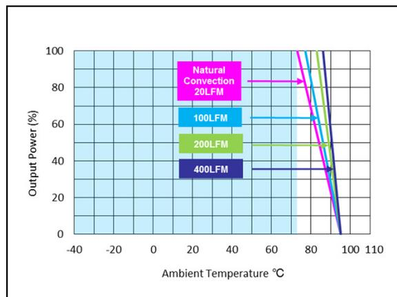
Figure 90: AEE01C48-M Derating Curve (without heatsink)
