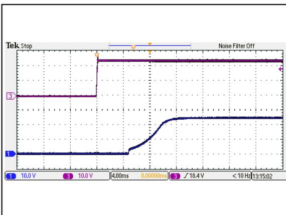
Figure 59: AEE01H24-M Output Voltage Startup Characteristic by Vin
