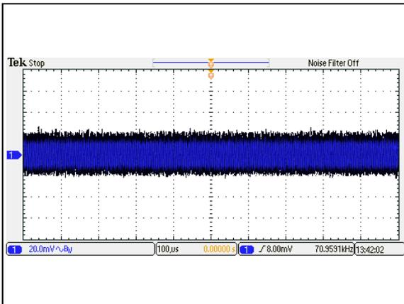
Figure 39: AEE03A24-M Ripple and Noise Measurement
