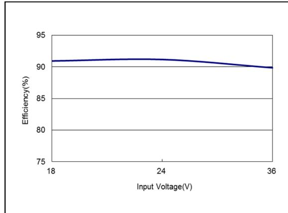
Figure 68: AEE01CC24-M Efficiency Versus Input Voltage Curve
