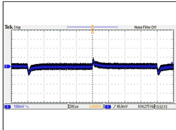
Figure 40: AEE03A24-M Transient Response
