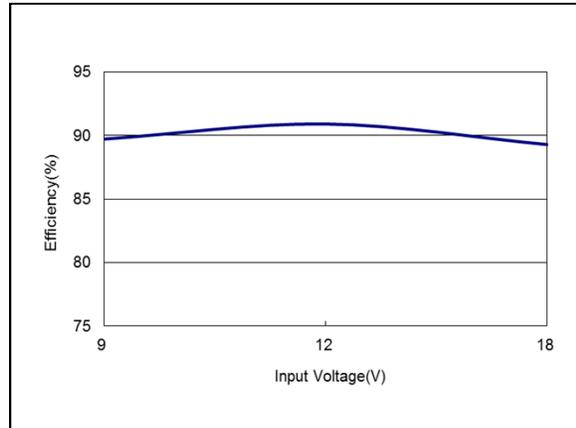
Figure 26: AEE01BB12-M Efficiency Versus Input Voltage Curve
