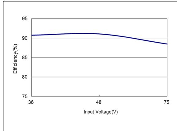
Figure 98: AEE01BB48-M Efficiency Versus Input Voltage Curve
