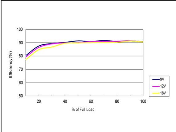
Figure 7: AEE01B12-M Efficiency Versus Output Current Curve
