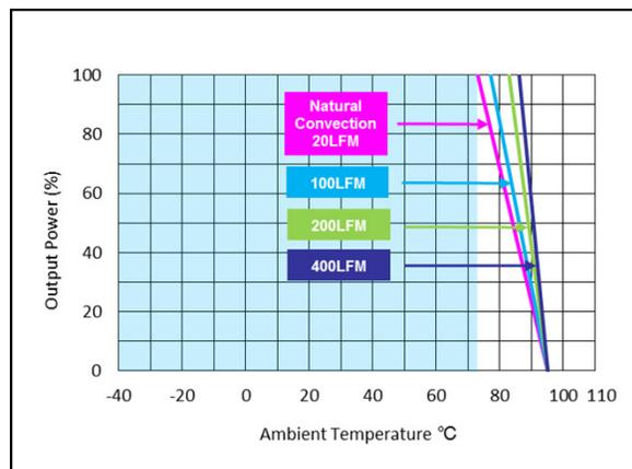
Figure 60: AEE01H24-M Derating Curve (without heatsink)
