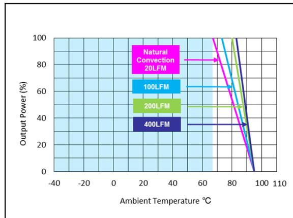
Figure 30: AEE01BB12-M Derating Curve (without heatsink)
