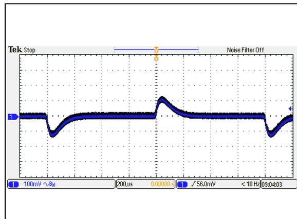
Figure 46: AEE01B24-M Transient Response
