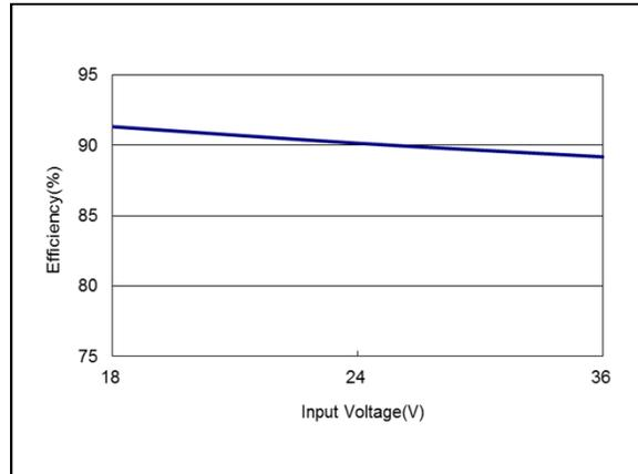
Figure 50: AEE01C24-M Efficiency Versus Input Voltage Curve
