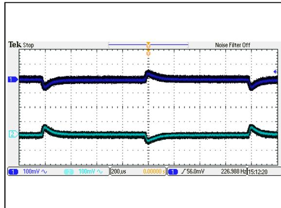
Figure 34: AEE01CC12-M Transient Response
