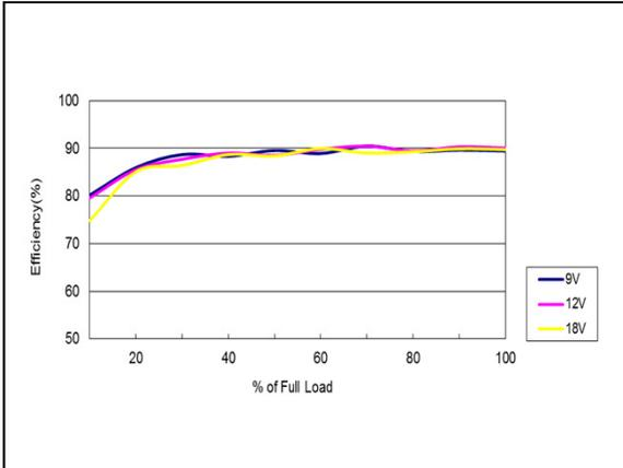
Figure 19: AEE01H12-M Efficiency Versus Output Current Curve
