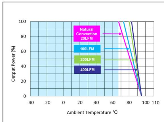
Figure 24: AEE01H12-M Derating Curve (without heatsink)
