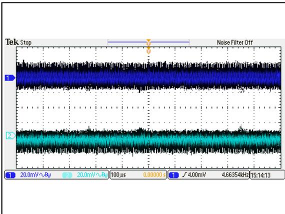
Figure 69: AEE01CC24-M Ripple and Noise Measurement
