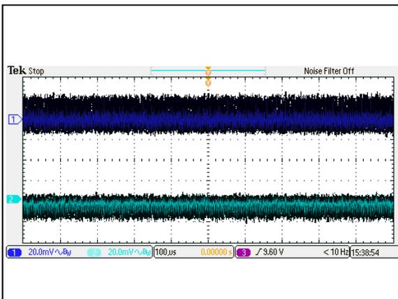
Figure 63: AEE01BB24-M Ripple and Noise Measurement
