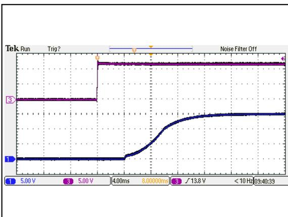
Figure 17: AEE01C12-M Output Voltage Startup Characteristic by Vin
