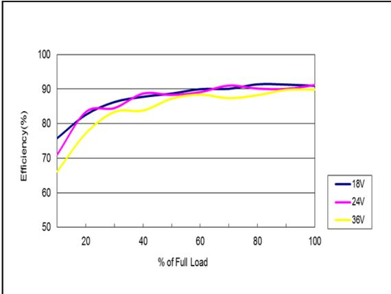
Figure 67: AEE01CC24-M Efficiency Versus Output Current Curve
