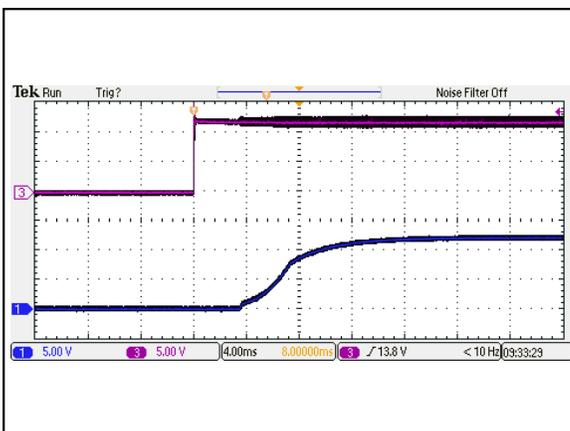
Figure 11: AEE01B12-M Output Voltage Startup Characteristic by Vin
