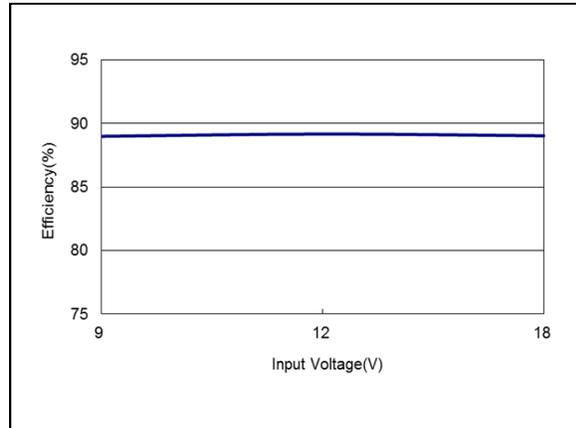
Figure 14: AEE01C12-M Efficiency Versus Input Voltage Curve
