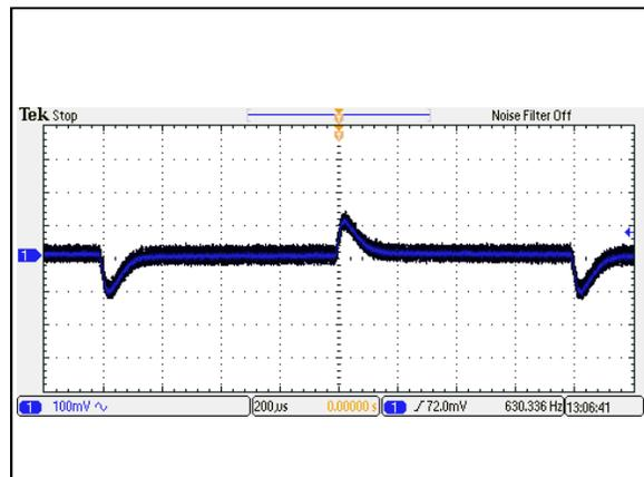
Figure 58: AEE01H24-M Transient Response
