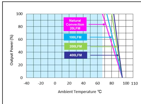
Figure 42: AEE03A24-M Derating Curve (without heatsink)
