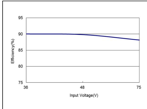
Figure 104: AEE01CC48-M Efficiency Versus Input Voltage Curve
