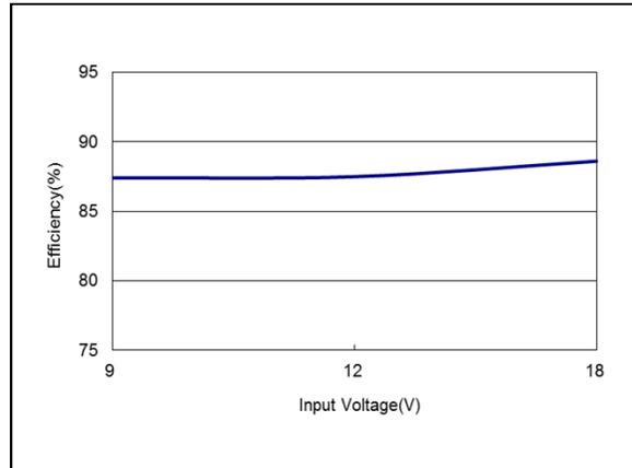
Figure 2: AEE03A12-M Efficiency Versus Input Voltage Curve
