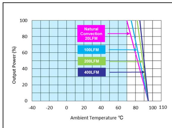
Figure 12: AEE01B12-M Derating Curve (without heatsink)
