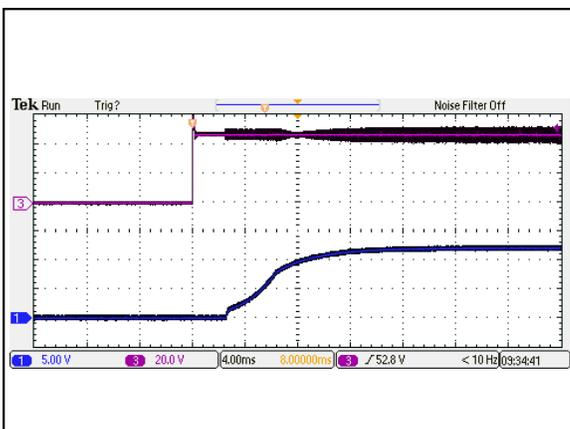
Figure 83: AEE01B48-M Output Voltage Startup Characteristic by Vin
