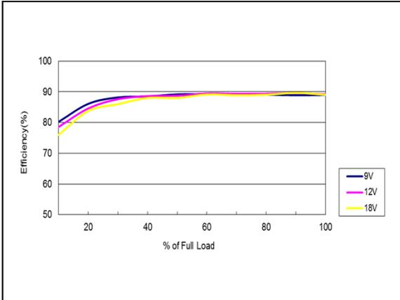
Figure 13: AEE01C12-M Efficiency Versus Output Current Curve
