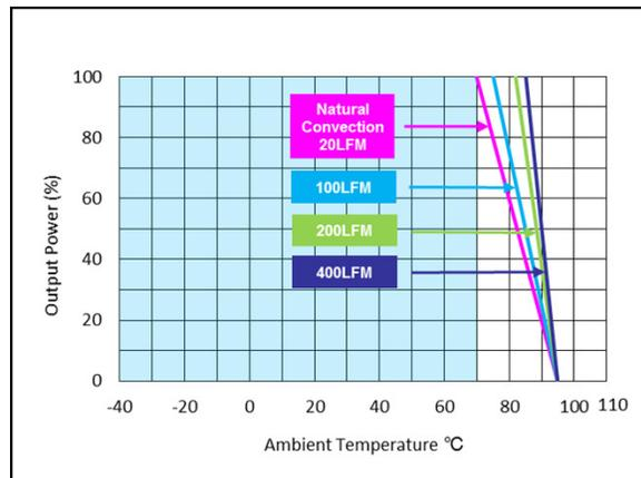
Figure 54: AEE01C24-M Derating Curve (without heatsink)
