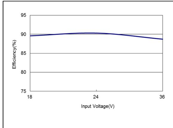
Figure 38: AEE03A24-M Efficiency Versus Input Voltage Curve
