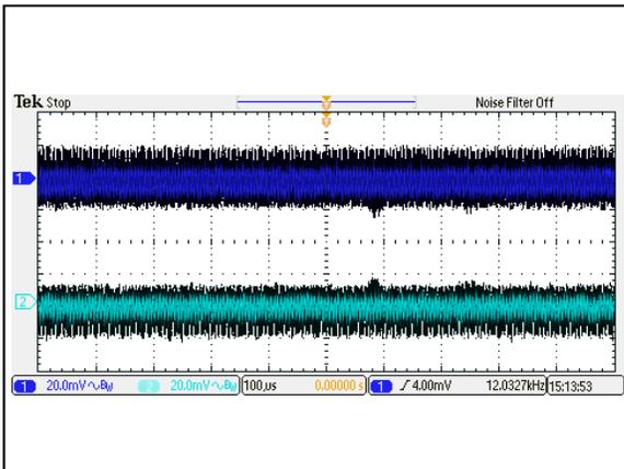
Figure 33: AEE01CC12-M Ripple and Noise Measurement
