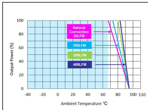
Figure 84: AEE01B48-M Derating Curve (without heatsink)
