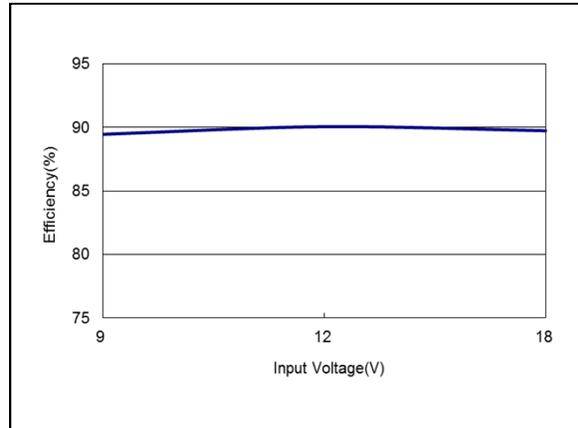
Figure 20: AEE01H12-M Efficiency Versus Input Voltage Curve
