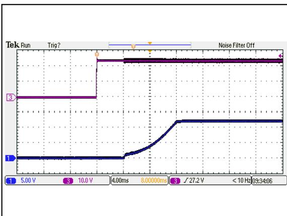
Figure 47: AEE01B24-M Output Voltage Startup Characteristic by Vin
