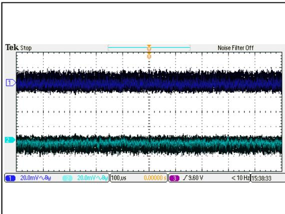
Figure 27: AEE01BB12-M Ripple and Noise Measurement
