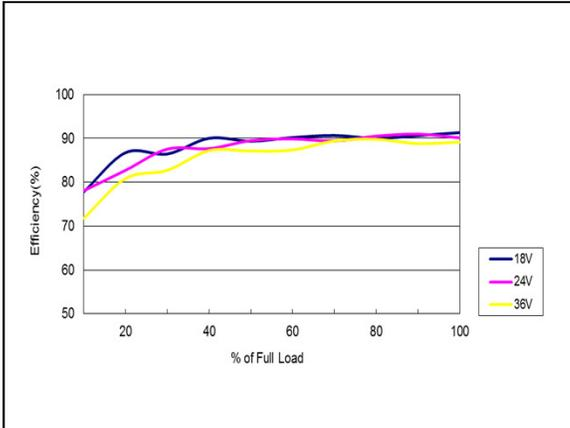
Figure 49: AEE01C24-M Efficiency Versus Output Current Curve
