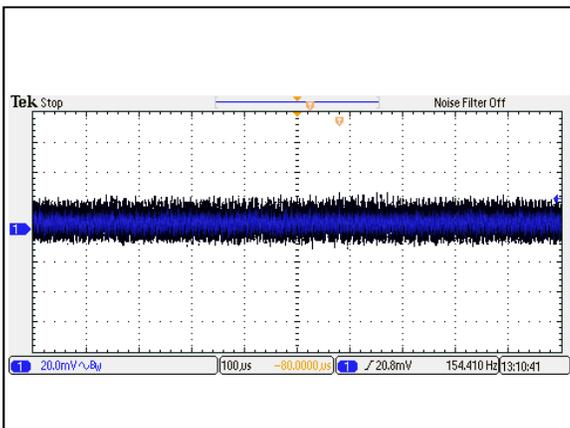
Figure 57: AEE01H24-M Ripple and Noise Measurement
