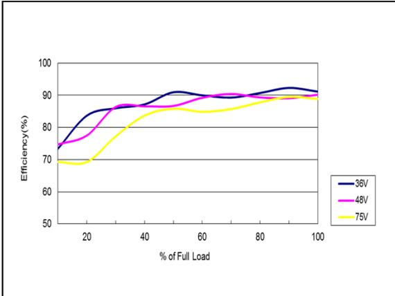
Figure 91: AEE01H48-M Efficiency Versus Output Current Curve
