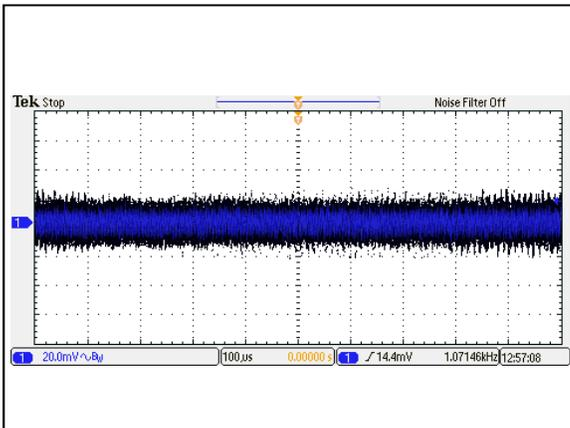
Figure 87: AEE01C48-M Ripple and Noise Measurement
