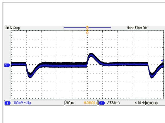
Figure 82: AEE01B48-M Transient Response
