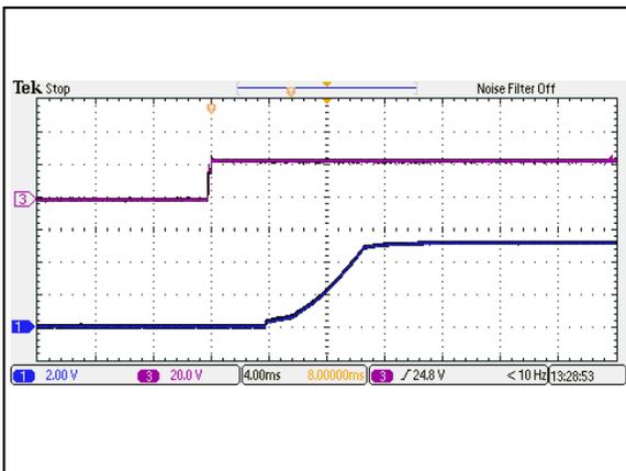
Figure 41: AEE03A24-M Output Voltage Startup Characteristic by Vin
