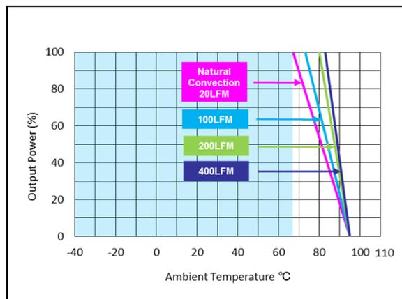
Figure 18: AEE01C12-M Derating Curve (without heatsink)
