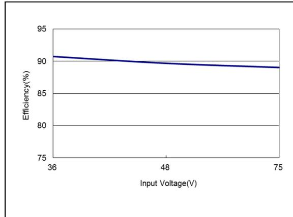
Figure 80: AEE01B48-M Efficiency Versus Input Voltage Curve
