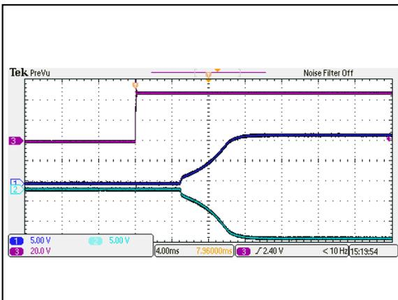
Figure 101: AEE01BB48-M Output Voltage Startup Characteristic by Vin
