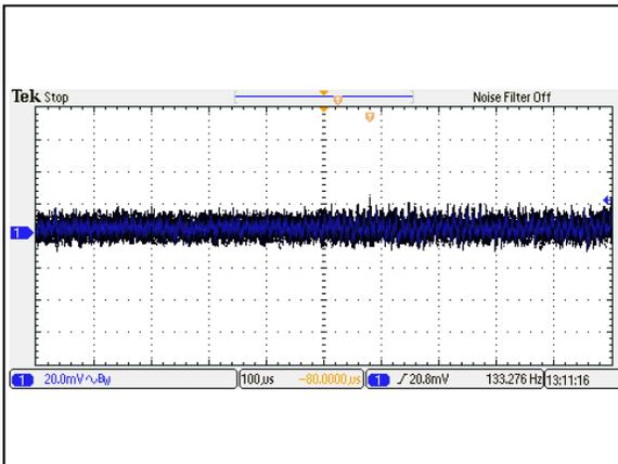
Figure 21: AEE01H12-M Ripple and Noise Measurement
