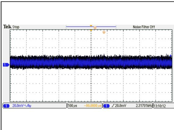
Figure 93: AEE01H48-M Ripple and Noise Measurement
