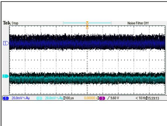
Figure 99: AEE01BB48-M Ripple and Noise Measurement
