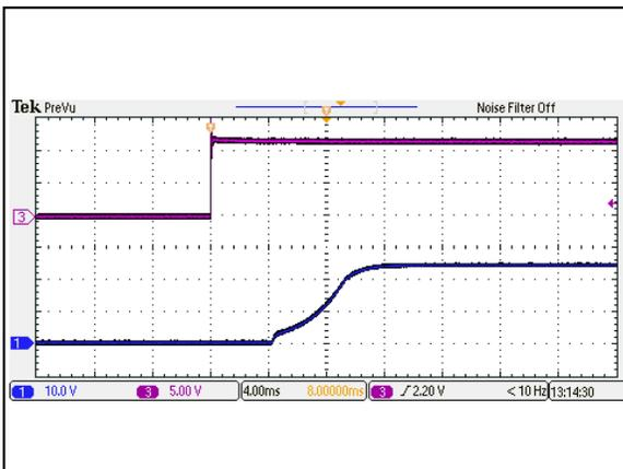
Figure 23: AEE01H12-M Output Voltage Startup Characteristic by Vin
