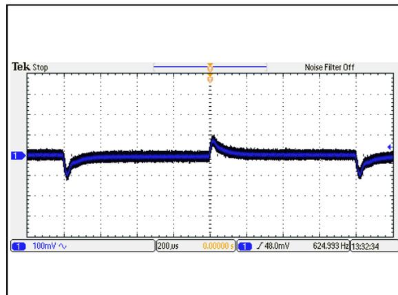
Figure 4: AEE03A12-M Transient Response
