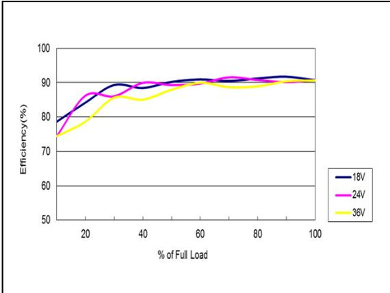
Figure 55: AEE01H24-M Efficiency Versus Output Current Curve
