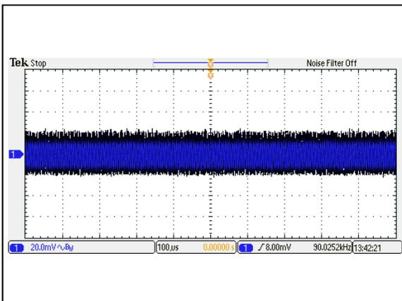
Figure 75: AEE03A48-M Ripple and Noise Measurement
