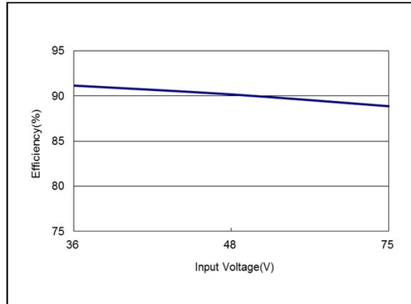
Figure 92: AEE01H48-M Efficiency Versus Input Voltage Curve
