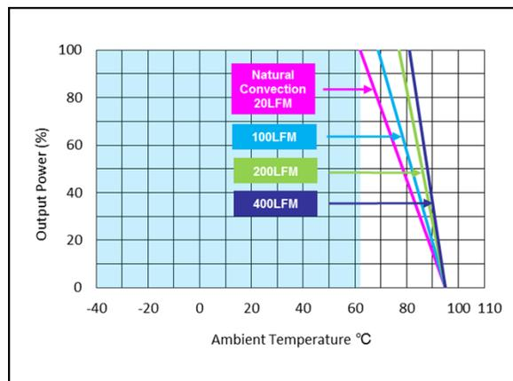
Figure 6: AEE03A12-M Derating Curve (without heatsink)
