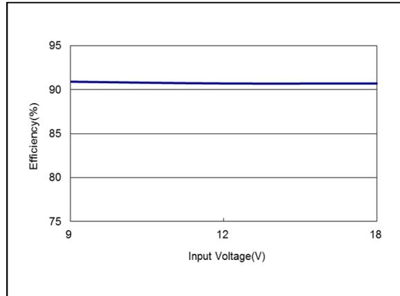
Figure 8: AEE01B12-M Efficiency Versus Input Voltage Curve
