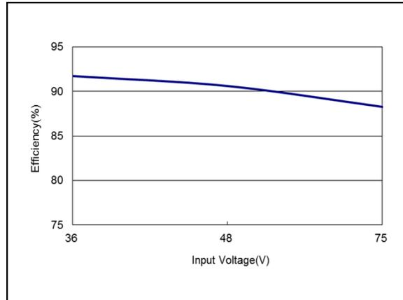
Figure 86: AEE01C48-M Efficiency Versus Input Voltage Curve
