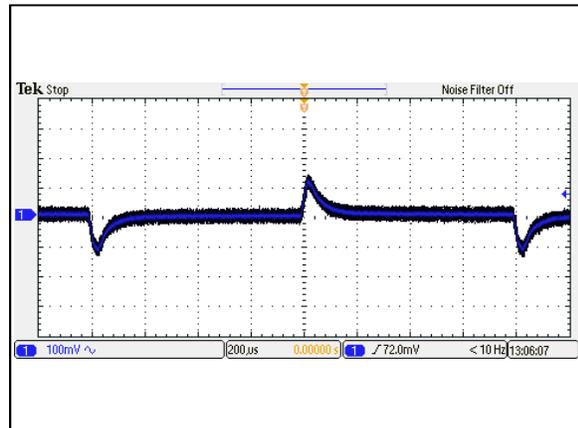
Figure 22: AEE01H12-M Transient Response
