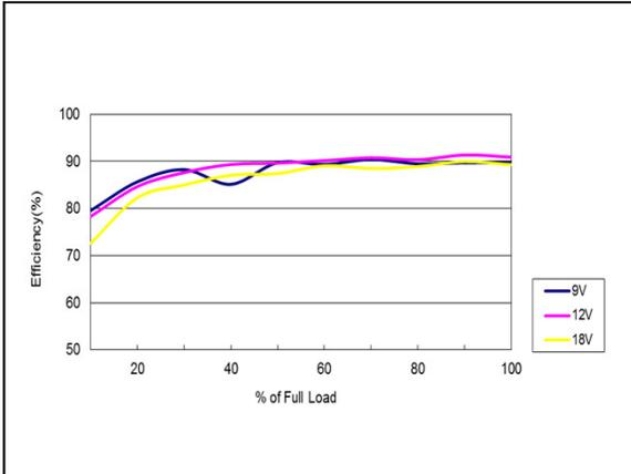
Figure 25: AEE01BB12-M Efficiency Versus Output Current Curve
