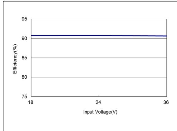
Figure 56: AEE01H24-M Efficiency Versus Input Voltage Curve
