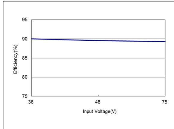
Figure 74: AEE03A48-M Efficiency Versus Input Voltage Curve
