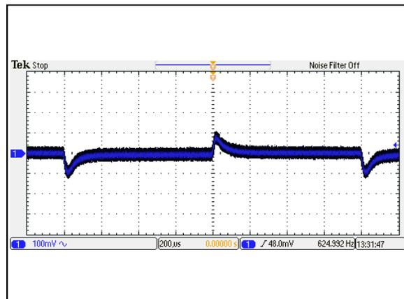
Figure 76: AEE03A48-M Transient Response
