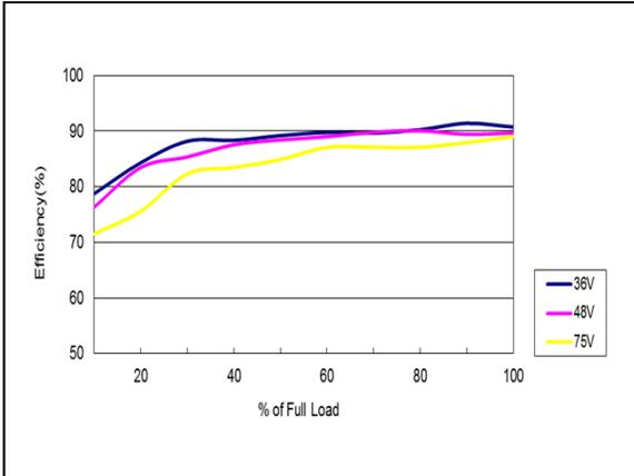
Figure 79: AEE01B48-M Efficiency Versus Output Current Curve
