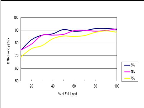
Figure 97: AEE01BB48-M Efficiency Versus Output Current Curve
