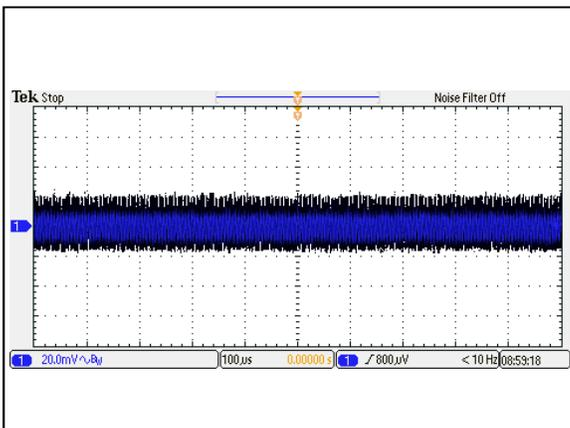
Figure 45: AEE01B24-M Ripple and Noise Measurement
