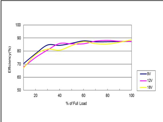
Figure 1: AEE03A12-M Efficiency Versus Output Current Curve
