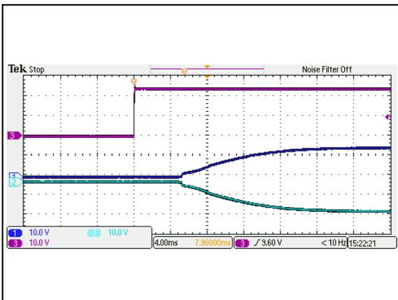
Figure 71: AEE01CC24-M Output Voltage Startup Characteristic by Vin
