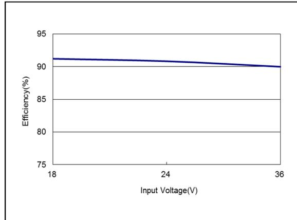
Figure 44: AEE01B24-M Efficiency Versus Input Voltage Curve
