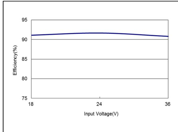
Figure 62: AEE01BB24-M Efficiency Versus Input Voltage Curve
