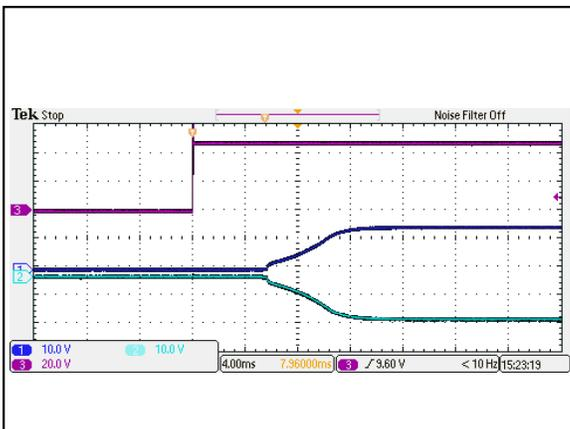
Figure 106: AEE01CC48-M Output Voltage Startup Characteristic by Vin
