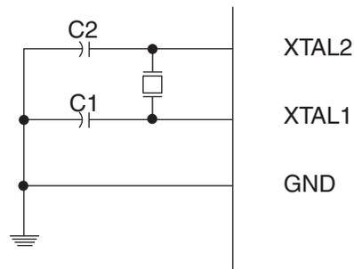
The Oscillator can operate in three different modes, each optimized for a specific frequency range. The operating mode is selected by the fuses CKSEL3..1 as shown in [Table 9-3 on page 28](#).
