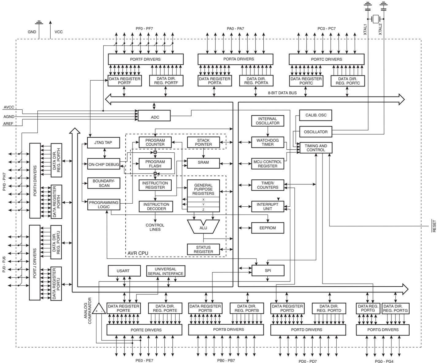
The Atmel®AVR® core combines a rich instruction set with 32 general purpose working registers. All the 32 registers are directly connected to the Arithmetic Logic Unit (ALU), allowing two independent registers to be accessed in one single instruction executed in one clock cycle. The
