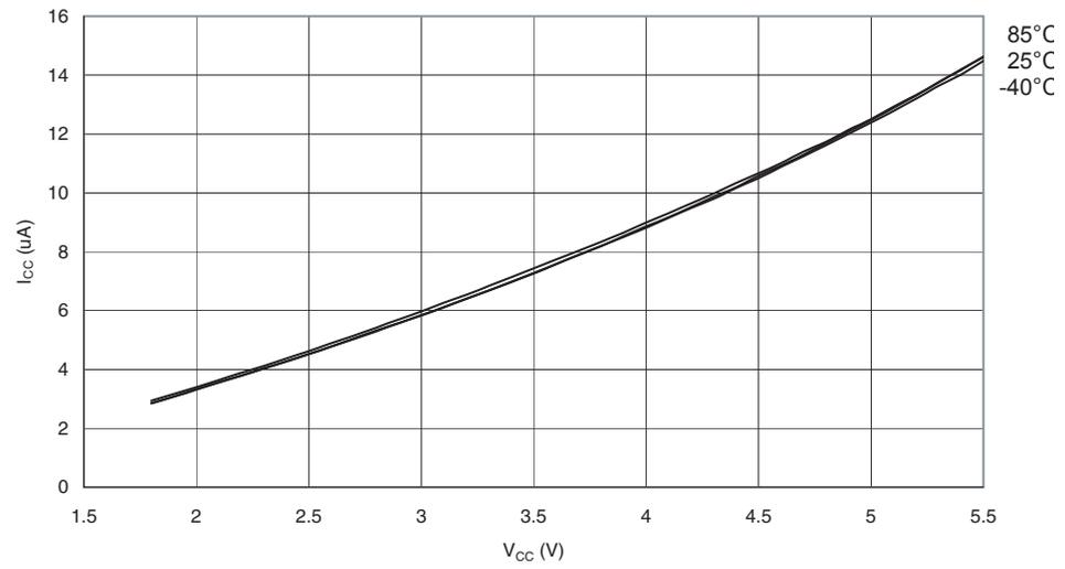
**Figure 29-54.** Analog Comparator Current vs.  $V_{CC}$
