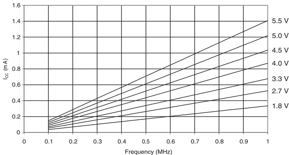
**Figure 29-2.** Active Supply Current vs. Frequency (1 - 16MHz)
