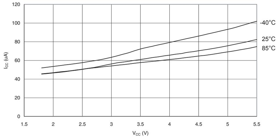
**Figure 29-55.** Programming Current vs.  $V_{CC}$
