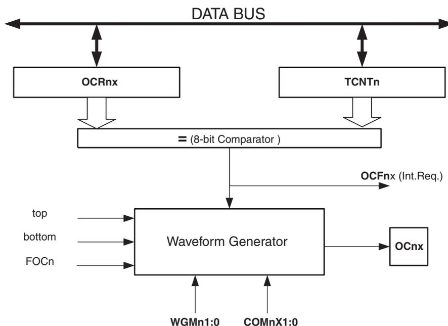
The OCR0A Register is double buffered when using any of the Pulse Width Modulation (PWM) modes. For the normal and Clear Timer on Compare (CTC) modes of operation, the double buffering is disabled. The double buffering synchronizes the update of the OCR0 Compare Register to either top or bottom of the counting sequence. The synchronization prevents the occurrence of odd-length, non-symmetrical PWM pulses, thereby making the output glitch-free.
