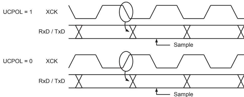
The UCPOLn bit in UCSRnC selects which XCK clock edge is used for data sampling and which is used for data change. As [Figure 20-3](#) shows, when UCPOLn is zero the data will be changed at rising XCK edge and sampled at falling XCK edge. If UCPOLn is set, the data will be changed at falling XCK edge and sampled at rising XCK edge.
