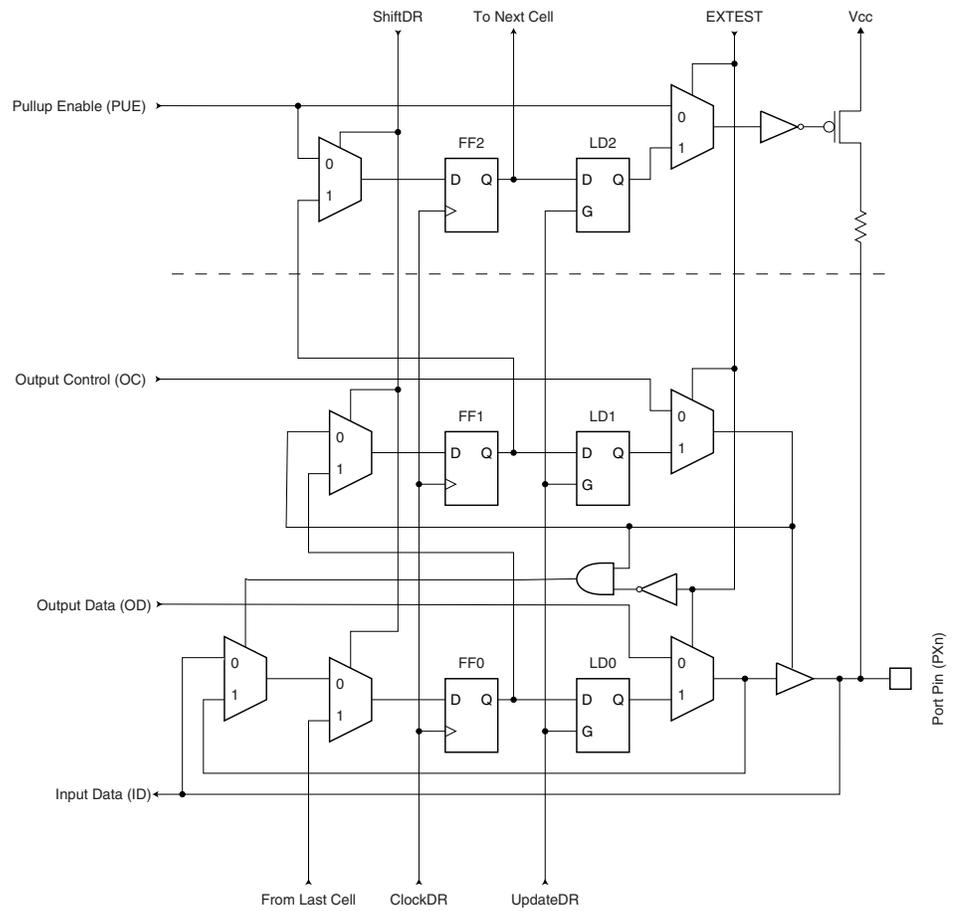
**Figure 25-4. General Port Pin Schematic Diagram**
