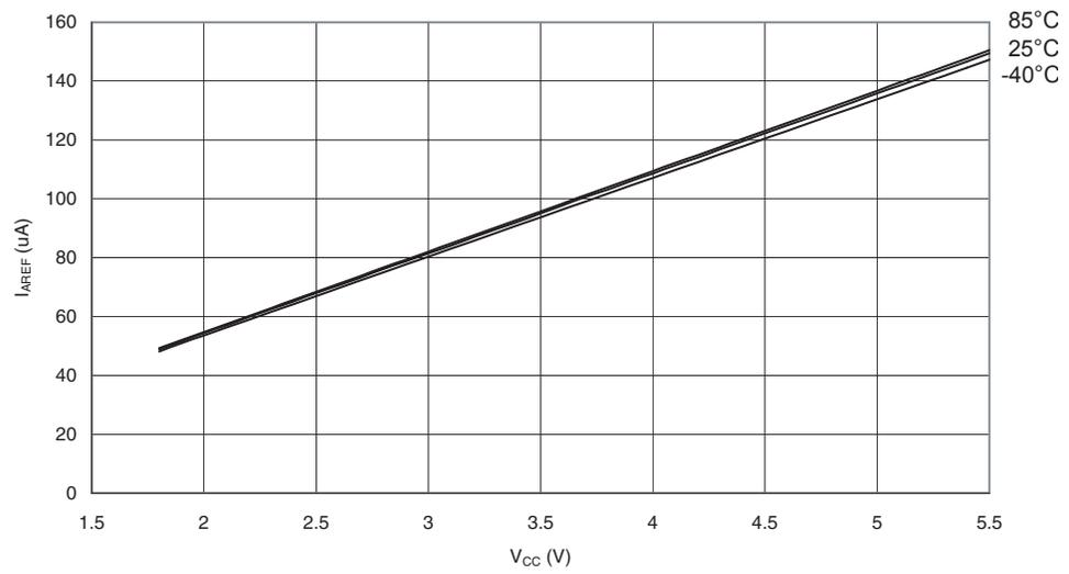
**Figure 29-52.** 32kHz TOSC Current vs.  $V_{CC}$  (Watchdog Timer Disabled)
