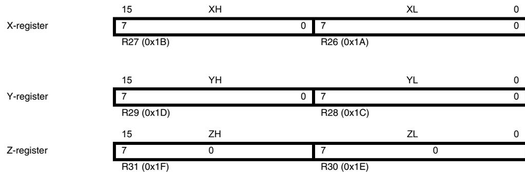
In the different addressing modes these address registers have functions as fixed displacement, automatic increment, and automatic decrement (see the instruction set reference for details).
