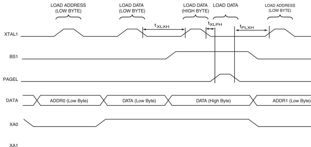
Note: 1. The timing requirements shown in [Figure 27-7](#) (i.e.,  $t_{DVXH}$ ,  $t_{XHL}$ , and  $t_{XLDX}$ ) also apply to loading operation.
