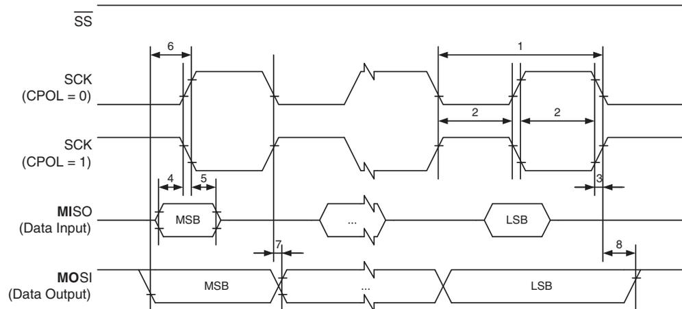
**Figure 28-5. SPI Interface Timing Requirements (Slave Mode)**
