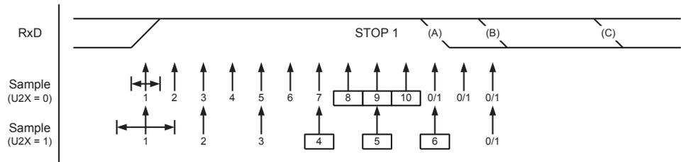
The same majority voting is done to the stop bit as done for the other bits in the frame. If the stop bit is registered to have a logic 0 value, the Frame Error (FEn) Flag will be set.
