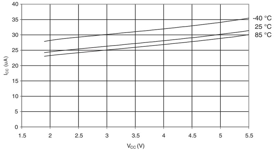
**Figure 29-50.** ADC Current vs.  $V_{CC}$  (AREF = AVCC)
