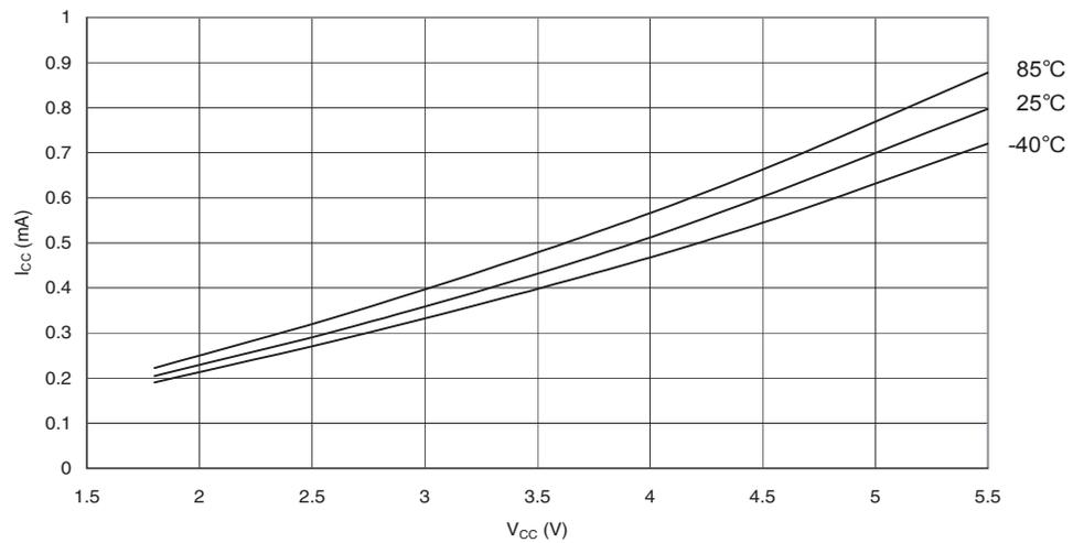
**Figure 29-10.** Idle Supply Current vs.  $V_{CC}$  (32kHz External Oscillator)
