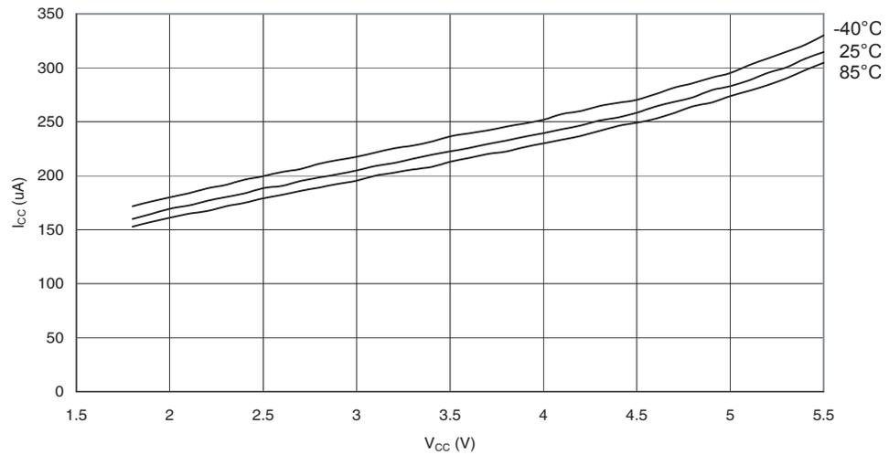
**Figure 29-51.** AREF External Reference Current vs.  $V_{CC}$
