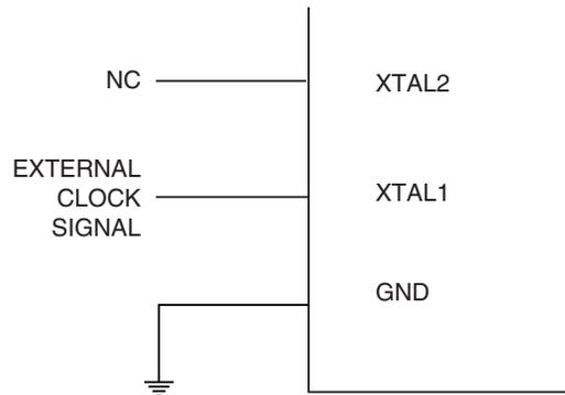
When this clock source is selected, start-up times are determined by the SUT Fuses as shown in [Table 9-10 on page 31](#).
