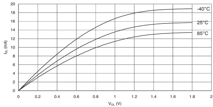
**Figure 29-29.** I/O Pin Sink Current vs. Output Voltage, Ports A, C, D, E, F, G, H, J ( $V_{CC} = 1.8V$ )
