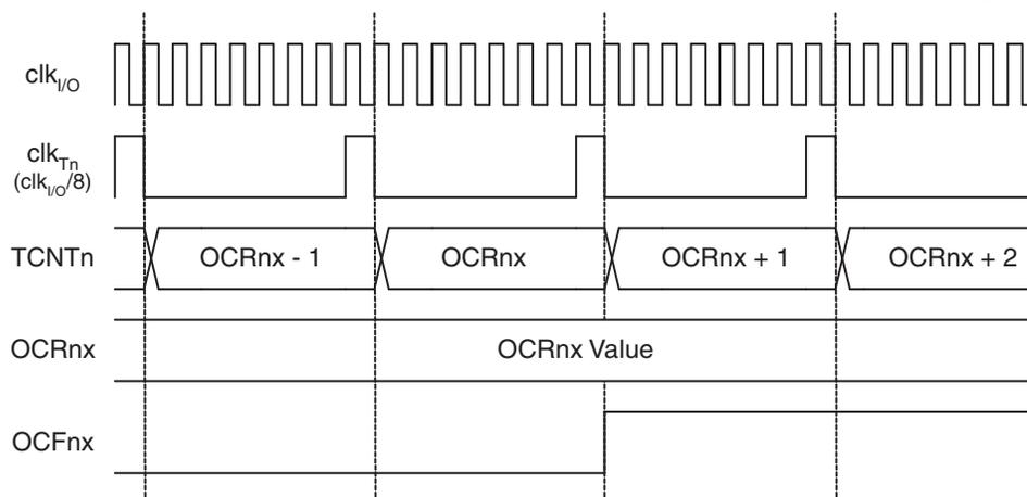
Figure 17-12 shows the count sequence close to TOP in various modes. When using phase and frequency correct PWM mode the  $OCR1x$  Register is updated at BOTTOM. The timing diagrams will be the same, but TOP should be replaced by BOTTOM, TOP-1 by BOTTOM+1 and so on. The same renaming applies for modes that set the TOV1 Flag at BOTTOM.
