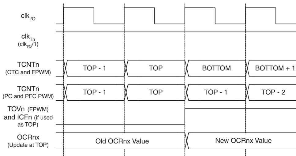
Figure 17-13 shows the same timing data, but with the prescaler enabled.
