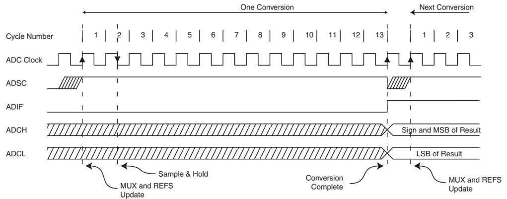
**Figure 23-6. ADC Timing Diagram, Auto Triggerred Conversion**
