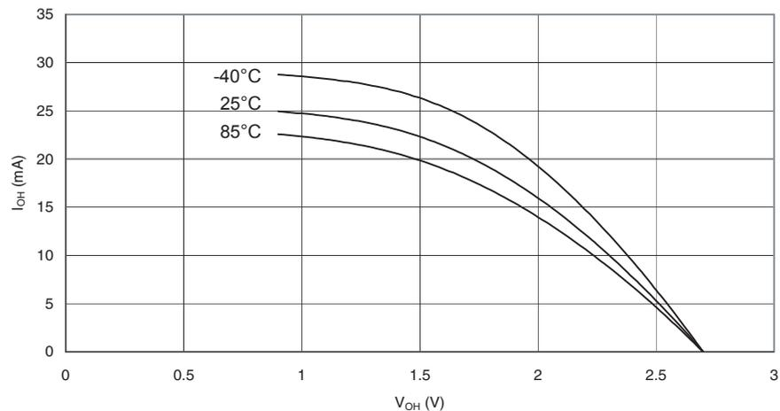
**Figure 29-26.** I/O Pin Source Current vs. Output Voltage, Port B ( $V_{CC} = 1.8V$ )
