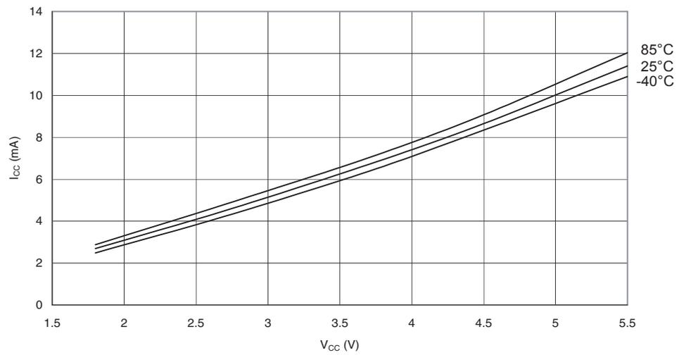
**Figure 29-4.** Active Supply Current vs.  $V_{CC}$  (Internal RC Oscillator, CKDIV8 Programmed, 1MHz)
