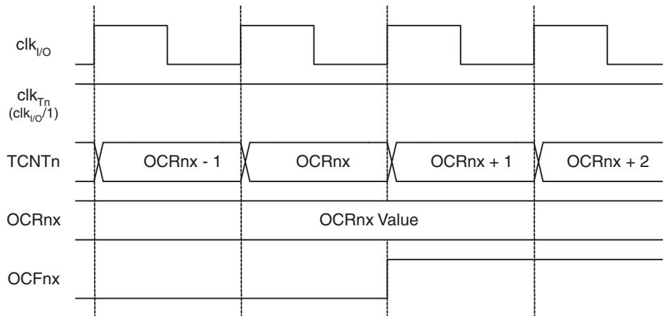
[Figure 17-11](#) shows the same timing data, but with the prescaler enabled.
