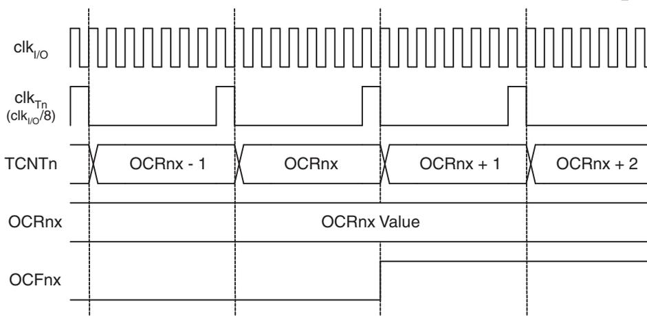
Figure 18-10 shows the setting of OCF2A and the clearing of TCNT2 in CTC mode.
