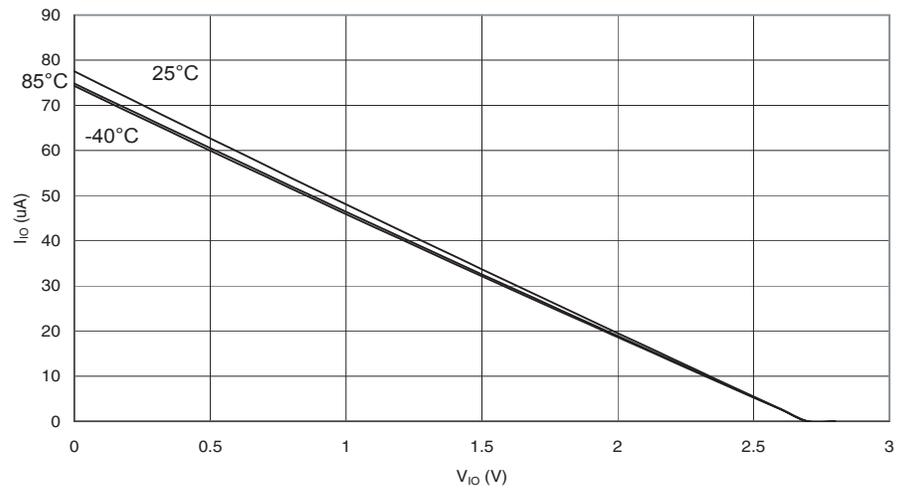
**Figure 29-17.** I/O Pin Pull-up Resistor Current vs. Input Voltage ( $V_{CC} = 1.8V$ )
