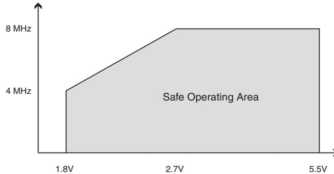
**Figure 28-2.** Maximum Frequency vs.  $V_{CC}$  (8 - 16 MHz).
