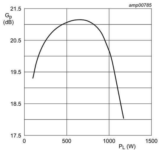
$V_{DS} = 50 \text{ V}$ ;  $I_{Dq} = 200 \text{ mA}$ ;  $t_p = 2.4 \text{ ms}$ ;  $\delta = 6.4 \text{ } \%$ .
