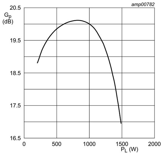
$V_{DS} = 50 \text{ V}$ ;  $I_{Dq} = 75 \text{ mA}$ ;  $t_p = 50 \text{ } \mu\text{s}$ ;  $\delta = 2 \text{ } \%$ .
