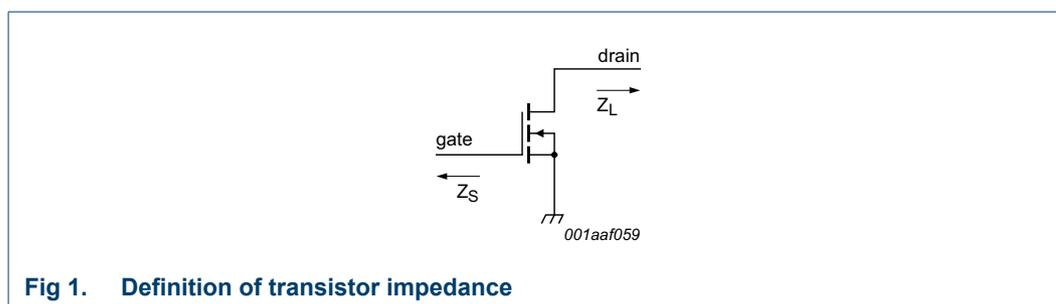
Fig 1. Definition of transistor impedance
