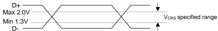
\*5: They indicate rising time (Trise) and falling time (Tfall) of the full-speed differential data signal.
