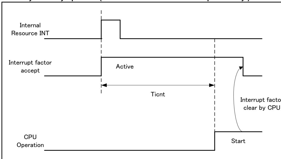
\*: Depending on the standby mode, interrupt from the internal resource is not included in the recovery cause.
