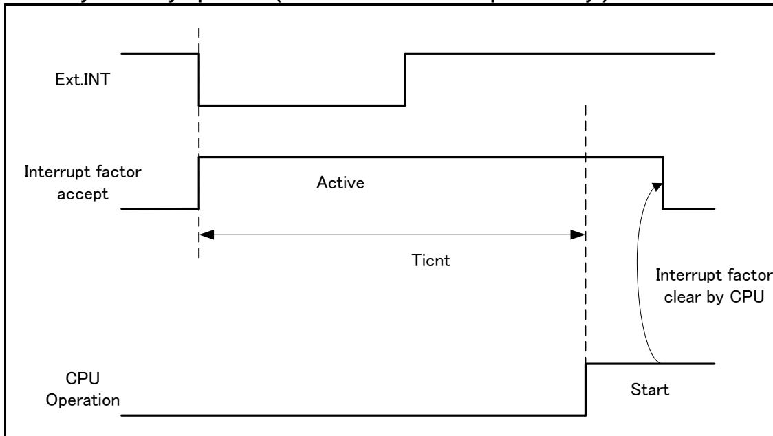
**Example of Standby Recovery Operation (when in Internal Resource Interrupt Recovery\*)**
