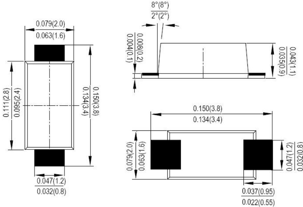
**Recommended Soldering Pattern (mm)**
