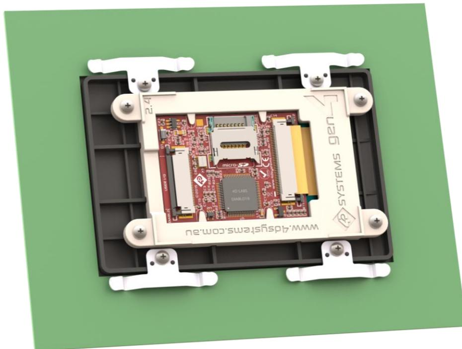
**Gen4-uLCD-24DT secured to the 2.4" Bezel, and Bezel secured to the Panel/Enclosure using the supplied small spring clips and screws**
