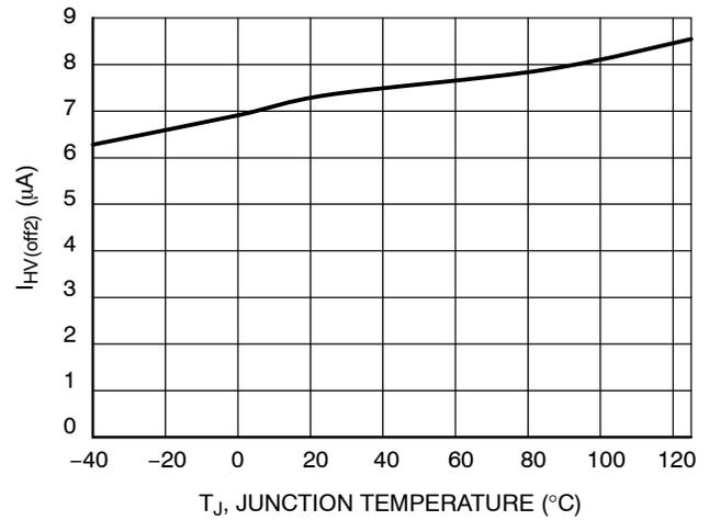
Figure 33. I<sub>HV(off2)</sub> vs. Temperature
