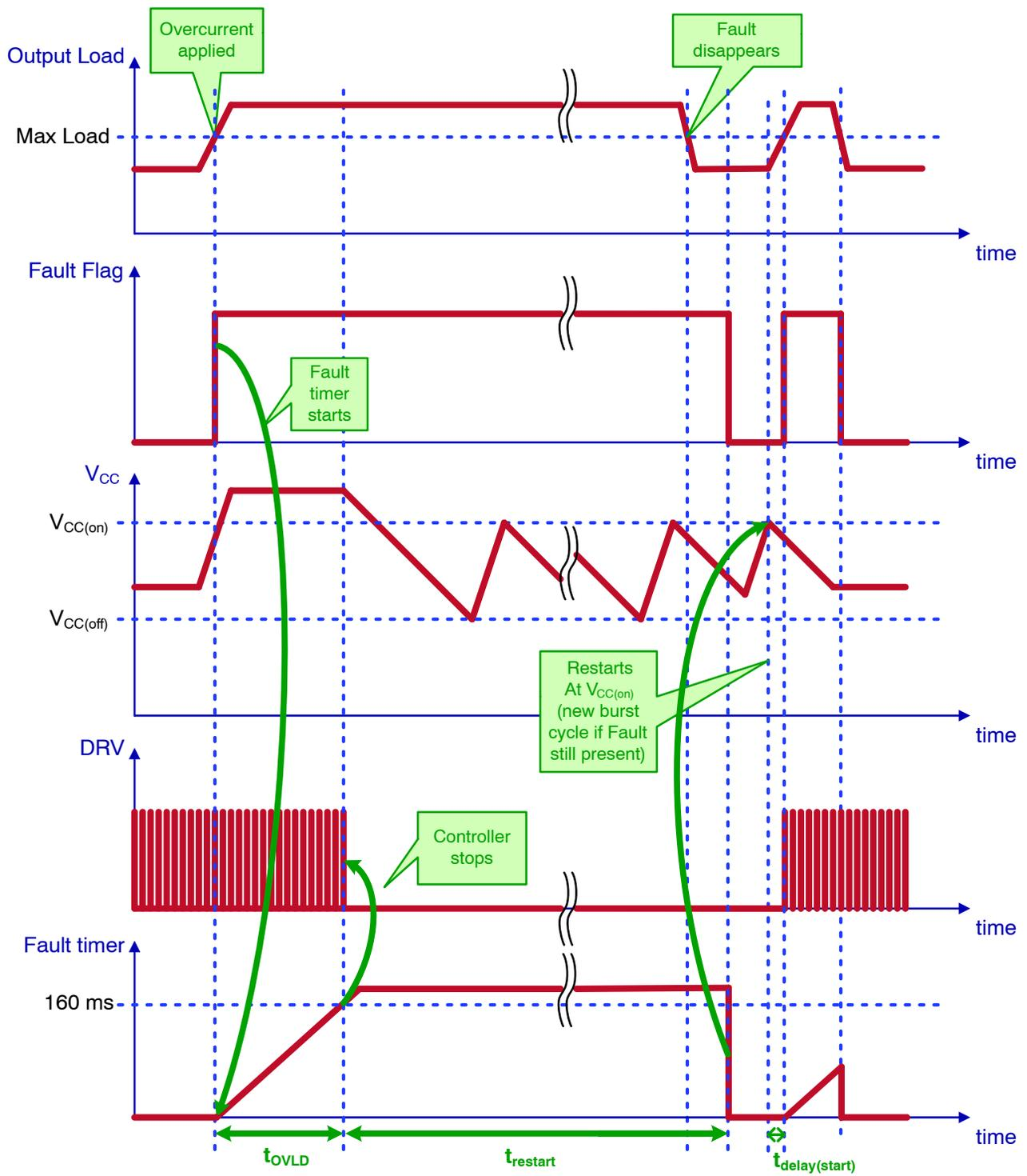
Figure 27. Auto-Recovery Overload Operation
