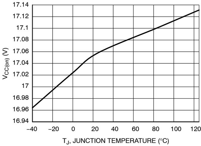
Figure 28. V<sub>CC(on)</sub> vs. Temperature
