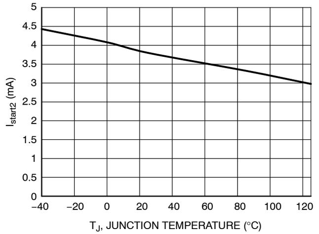
Figure 31. I<sub>start2</sub> vs. Temperature
