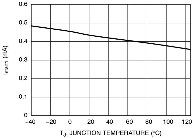
Figure 30. I<sub>start1</sub> vs. Temperature
