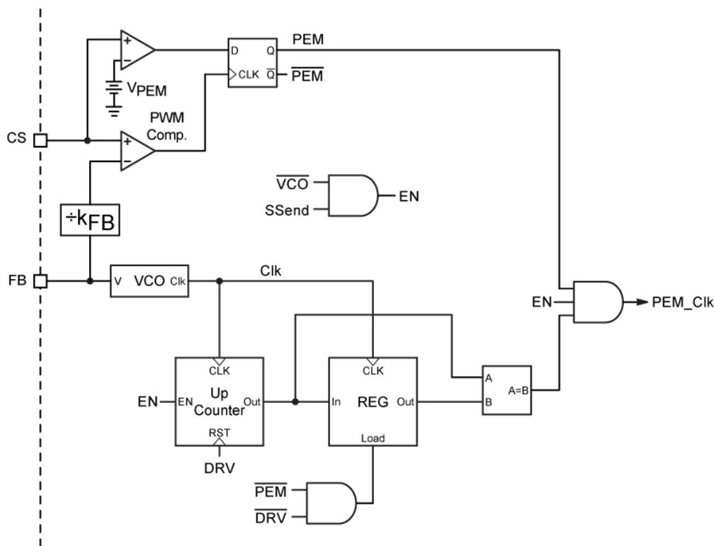
Figure 17. PEM Block Diagram
