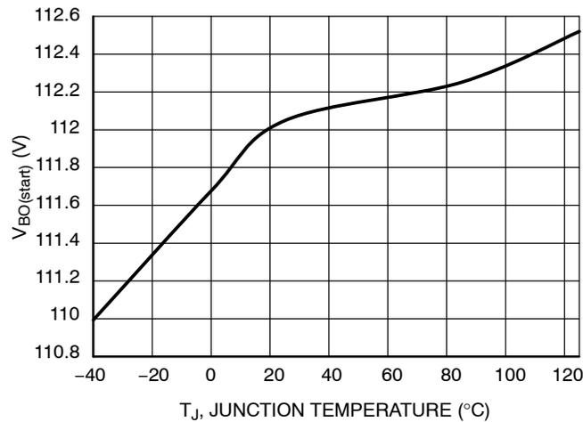
Figure 38. V<sub>BO(start)</sub> vs. Temperature
