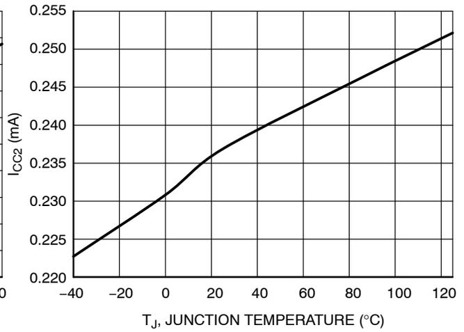
Figure 35. I<sub>CC2</sub> vs. Temperature
