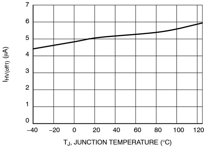
Figure 32. I<sub>HV(off1)</sub> vs. Temperature
