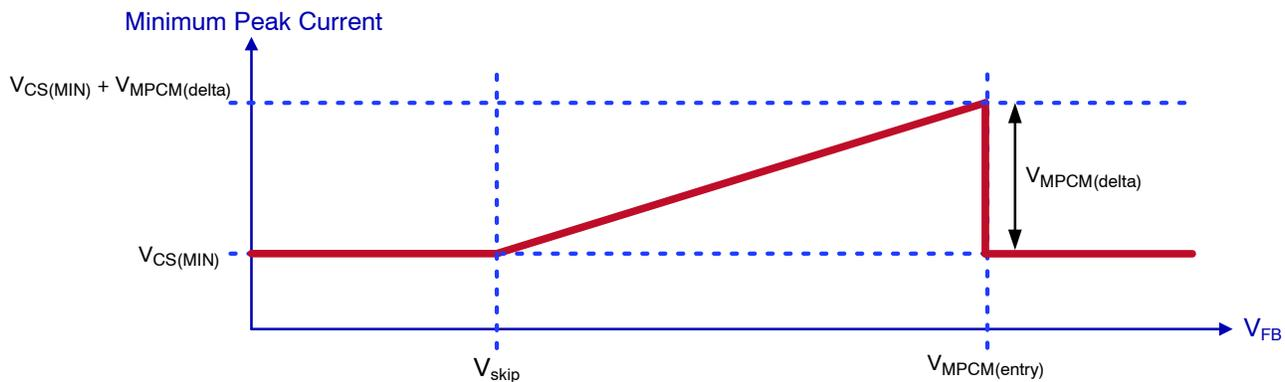
Figure 14. Minimum Peak Current Modulation
