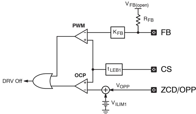
Figure 8. OPP Circuit Schematic
