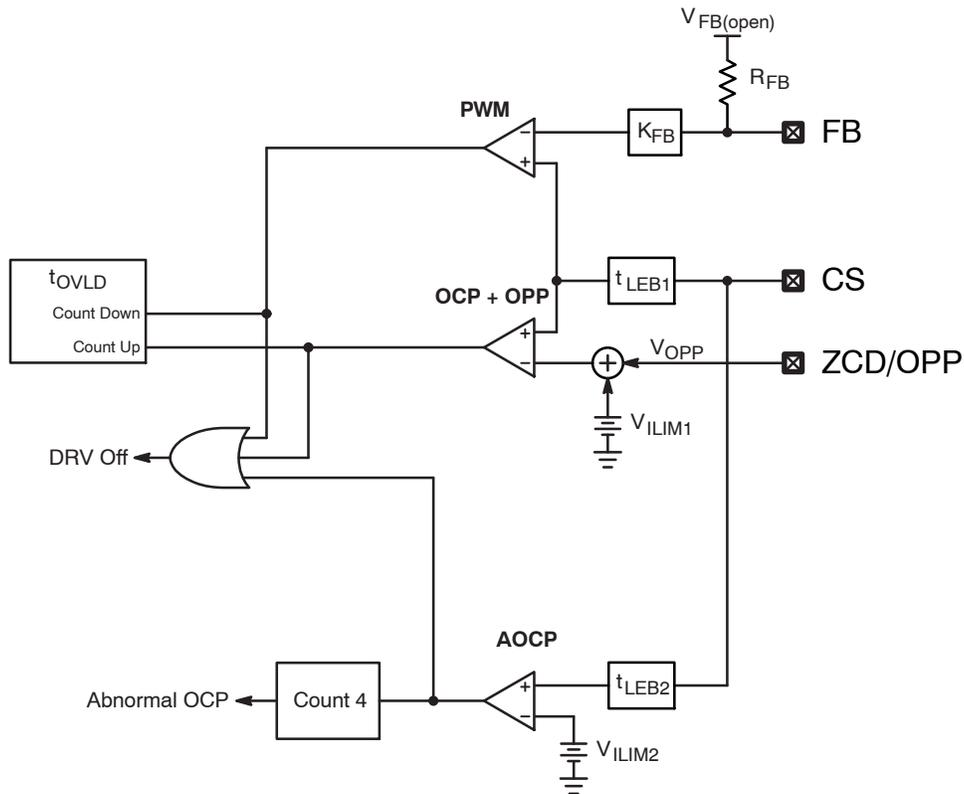
Figure 25. Overload Circuitry
