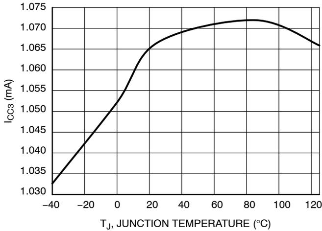
Figure 36. I<sub>CC3</sub> vs. Temperature
