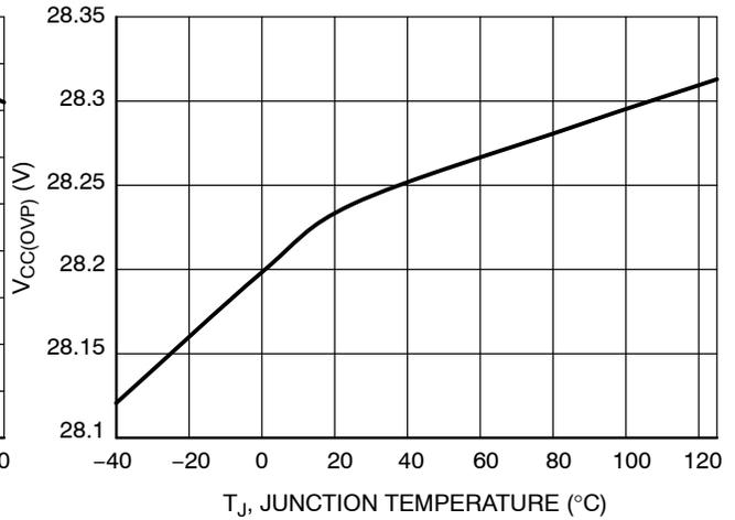
Figure 37. V<sub>CC(OVP)</sub> vs. Temperature
