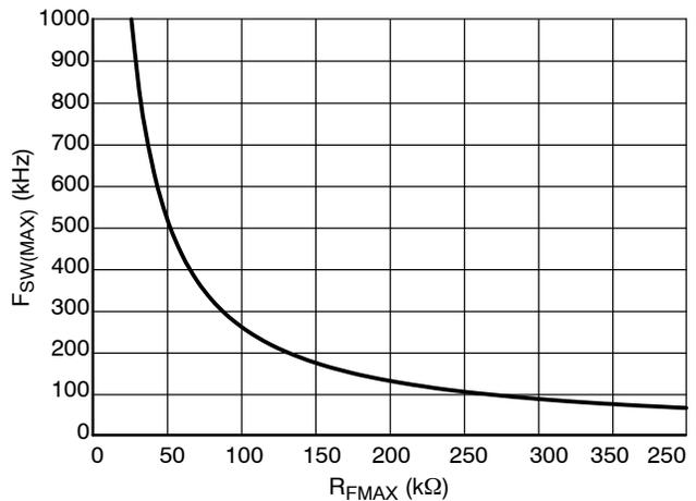
**Figure 11. F<sub>SW(MAX)</sub> vs. R<sub>FMAX</sub>**
