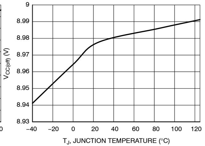
Figure 29. V<sub>CC(off)</sub> vs. Temperature
