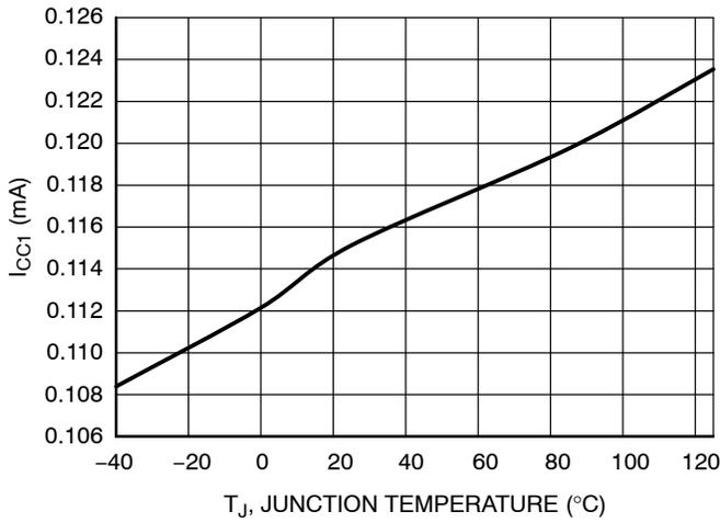
Figure 34. I<sub>CC1</sub> vs. Temperature
