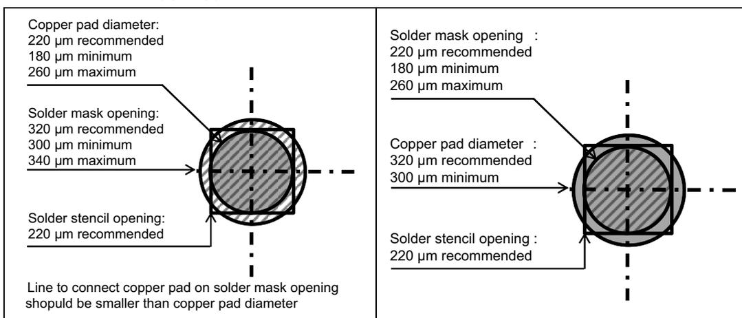
Figure 12. Marking specification
