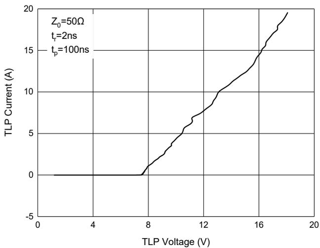
Fig. 6 - ESD Clamping Voltage
