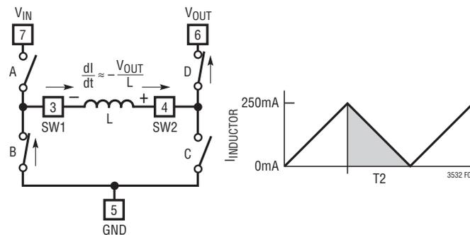
Figure 4. Inductor Discharge Cycle During Burst Mode Operation
