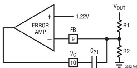
Figure 7. Error Amplifier with Type I Compensation
