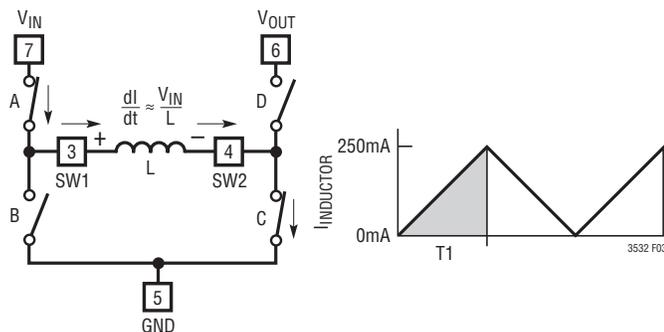
Figure 3. Inductor Charge Cycle During Burst Mode Operation
