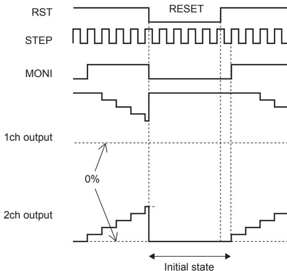
When the RST pin is set Low, the output excitation position is forced to the initial state, and the MONI output also goes Low.
