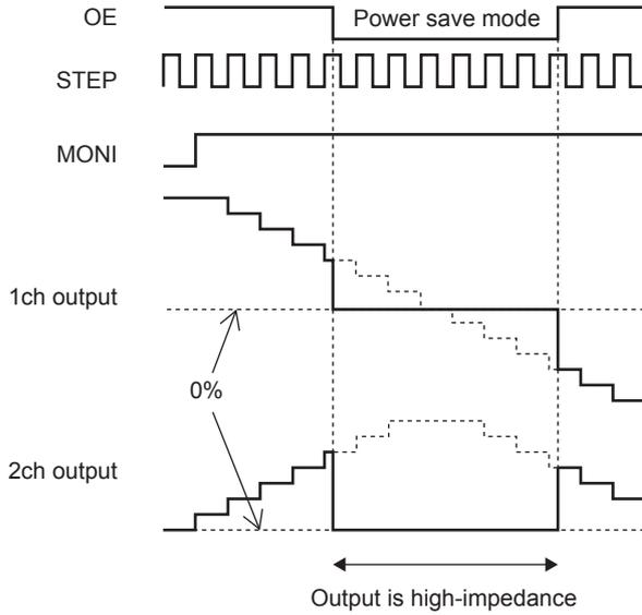
When the OE pin is set Low, the output is forced OFF and goes to high impedance. However, the internal logic circuits are operating, so the excitation position proceeds when the STEP signal is input. Therefore, when OE is returned to High, the output level conforms to the excitation position proceeded by the STEP input.
