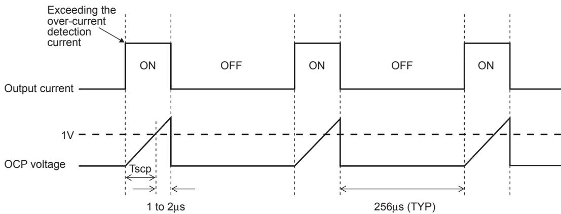
When detecting the output short-circuit state, the short-circuit detection circuit is activated. When the short-circuit detection circuit operation exceeds the timer latch time described later, the output is changed over to the standby mode and reset to the ON mode again in 256µs (TYP). In this event, if the overcurrent mode still continues, the above switching mode is repeated till the overcurrent mode is canceled.
