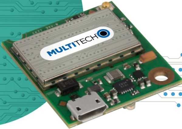
MultiTech Dragonfly™ Nano embedded cellular modems and SoMs are one of the industry's smallest form factor, end device approved, devices that can support a complete IoT operating system. The Dragonfly Nano is over 50% smaller, maintains plug compatibility and uses the same 40-pin board to board connector or USB connector found in the standard sized Dragonfly family; providing a full range of connectivity and carrier options.
