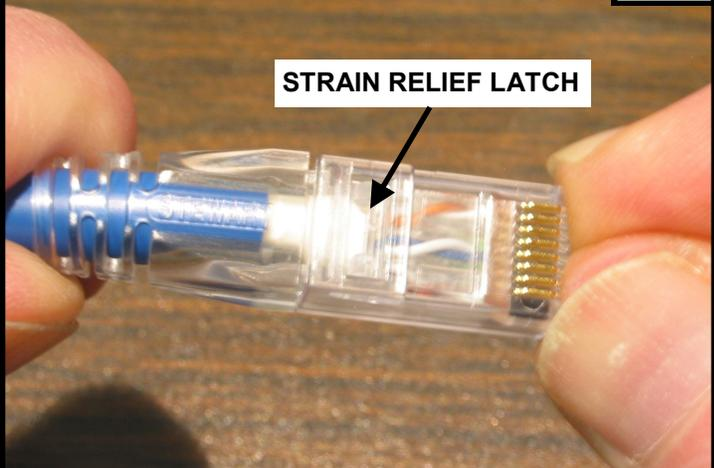
Push the plug body over the load bar, aligner and boot (if used). The jacket should extend under the strain relief latch and load bar should be tight against the front of the plug body.
