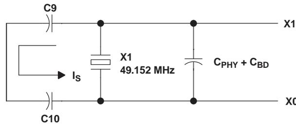
Figure 10. Load Capacitance for the TSB41BA3D PHY
