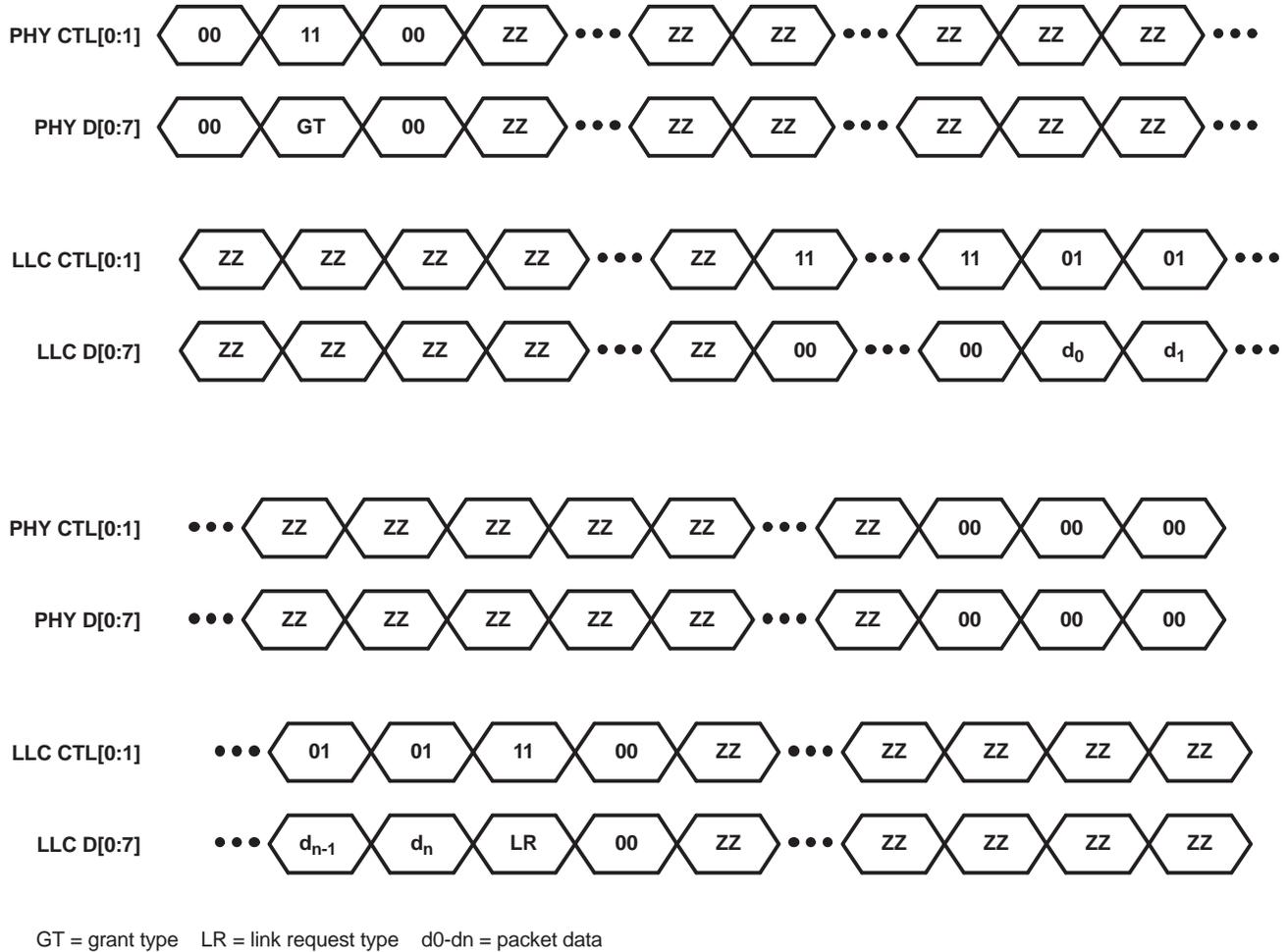
**Figure 29. Transmit Packet Timing With Optional Link Request**
